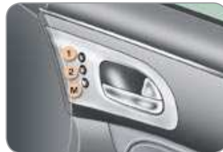
M. Adjustments memorisation. 1. Recall of the first position. 2. Recall of the second position.
