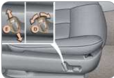
D. Seat back angle adjustment. E. Head restraint height adjustment.
