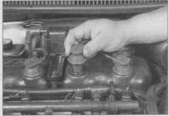
27.7b Use a twisting motion to free the boot and then pull it from the valve cover
