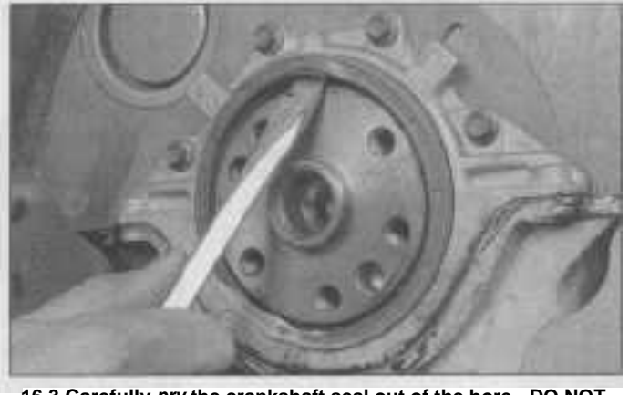
16.3 Carefully pry the crankshaft seal out of the bore - DO NOT nick or scratch the crankshaft or seal bore
