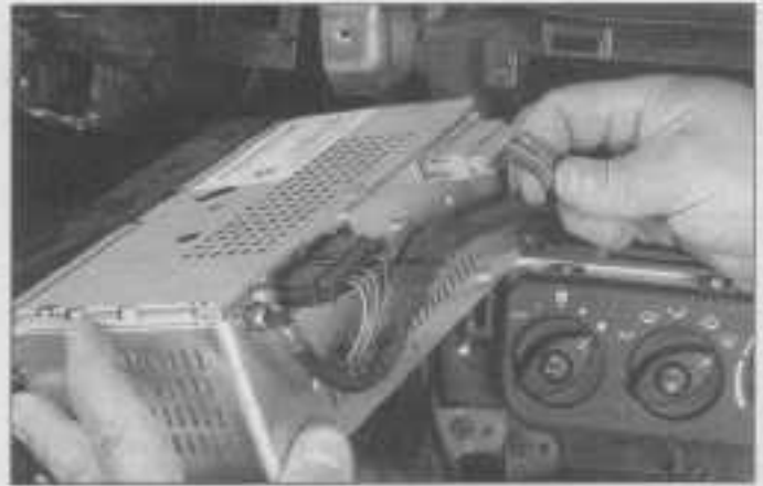
17.4 Disconnecting the electrical connectors and antenna lead from the rear of the radio
