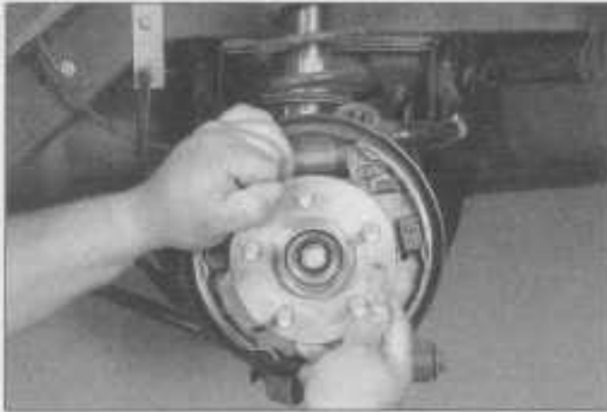
17.5 Pull the rear hub/bearing assembly off of the knuckle spindle
