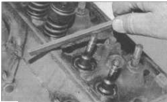
10.4c If the valve stem won't pass through the guide, chances are its because of a burr or raised material on the end of the valve stem. Use a fine file or whetstone to deburr the valve stem as required
