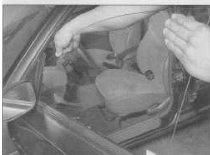
15.9 Carefully maneuver the glass out of the opening in the top of the door
