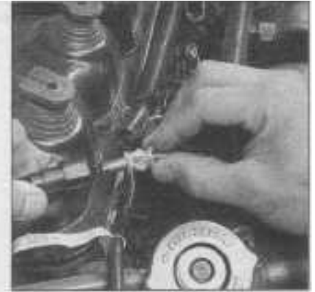
4.9b ... and separate the fitting - to assemble it, lubricate the male end with a small amount of clean engine oil, then push the fitting together until it locks into place - tug on it to ensure the connection is secure
