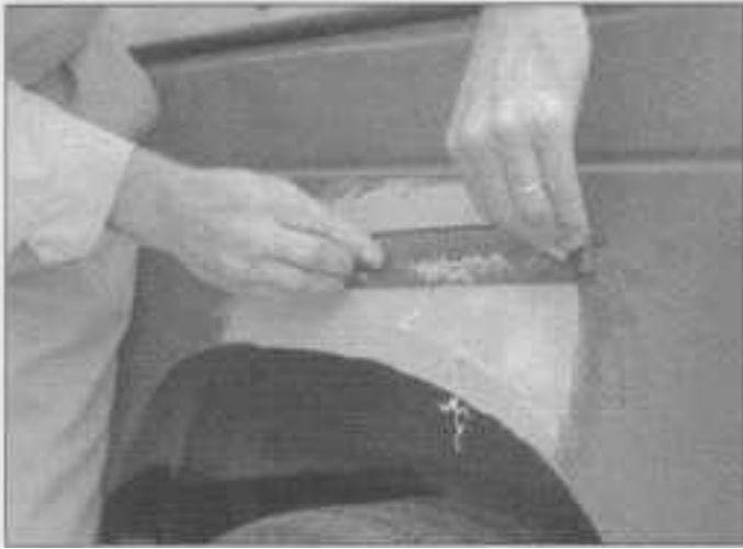
7 Let the filler harden until you can just dent it with your fingernail. Use a body file or Surform tool (shown here) to rough-shape the filler
