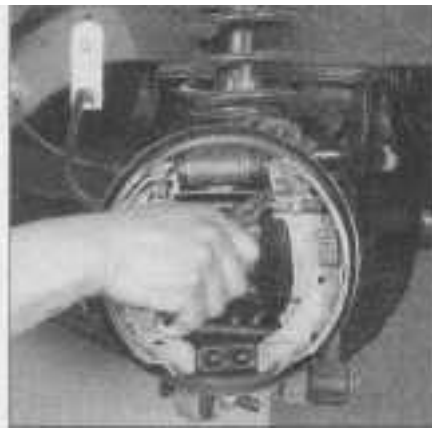
6.4c Using locking pliers, grasp the upper return spring and detach it from the trailing brake shoe
