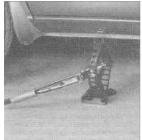
The jack fits over the rocker panel flange (there are two jacking points on each side of the vehicle, indicated by a notch in the rocker panel flange)
