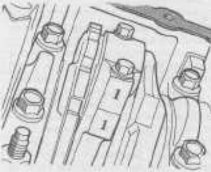
26.14 Install the connecting rod cap making sure the cap and rod identification numbers match
