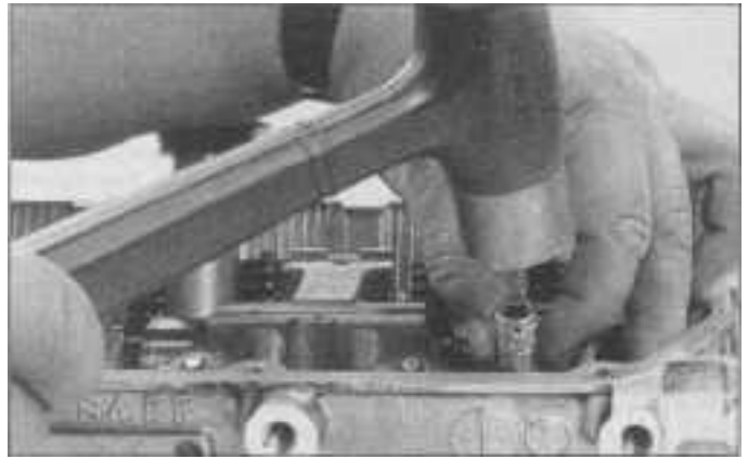
13.4b Install the valve stem seal using an appropriate size socket and hammer
