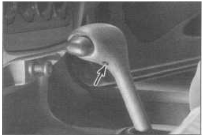
26.4 To remove the shift lever handle on vehicles equipped with an automatic transaxle, remove the set screw (arrow) and pull the handle off the shift lever
