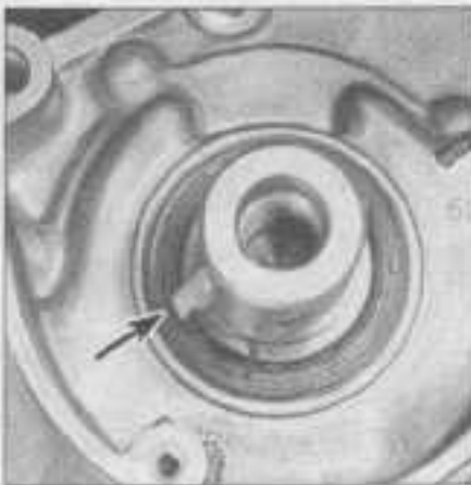
7.2 After removing the timing belt sprocket, remove the Woodruff key (arrow) from the crankshaft
