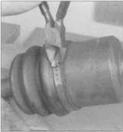
9.2 Cut the boot clamps and remove them from the driveaxle
