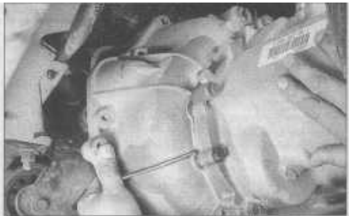
6.31 While removing the transaxle from the engine, make sure to keep it level so the modular clutch assembly doesn't fall off the transaxle input shaft
