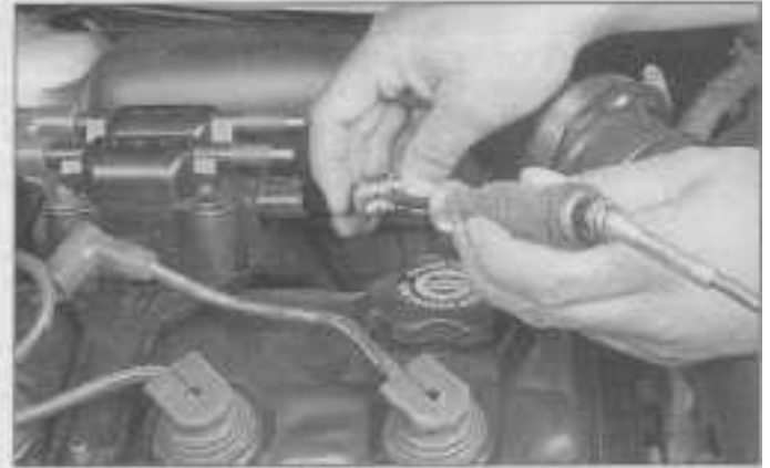
6.9 On four-cylinder engines, connect a test light between the coil electrical connector center terminal and one of the outer terminals. Crank the engine. The test light should blink on-and-off
