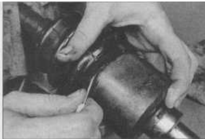
9.34 Equalize the pressure in the boot by inserting a small, dull screwdriver between the boot and the joint housing
