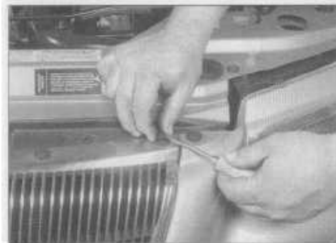
12.7 To remove the push-in fasteners, pry out the center stud and then remove the outer housing
