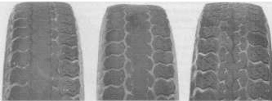
INCORRECT TOE-1N OR EXTREME CAMBER
