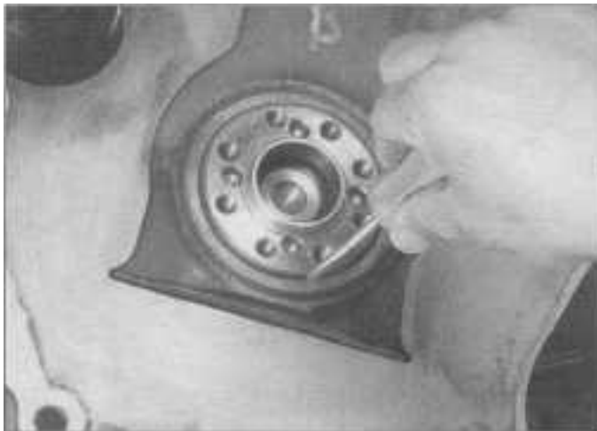
16.3 Using a 3/16 inch flat blade screwdriver, very carefully pry the crankshaft rear main seal out of its bore - DO NOT nick or scratch the sealing surfaces on the crankshaft or seal bore
