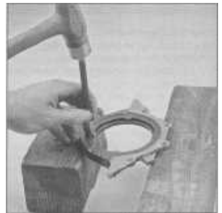
16.6 With the seal retainer supported on wood blocks, use a hammer and drift to drive the seal out of the retainer
