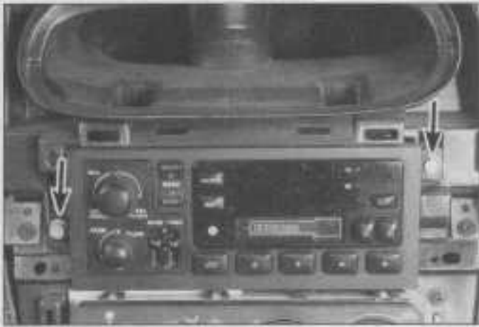
17.3 Radio mounting screws (arrows)
