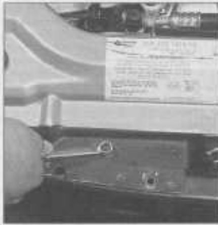
15.4 Remove the upper radiator support crossmember
