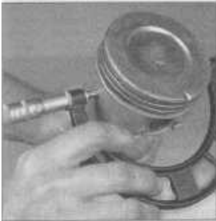
20.11 Measure the piston diameter 90 degrees from the piston pin and the specified distance from the bottom of the piston skirt
