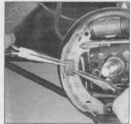
6.4s Compress the retaining clip and turn the pin 90-degrees to retain the brake shoe
