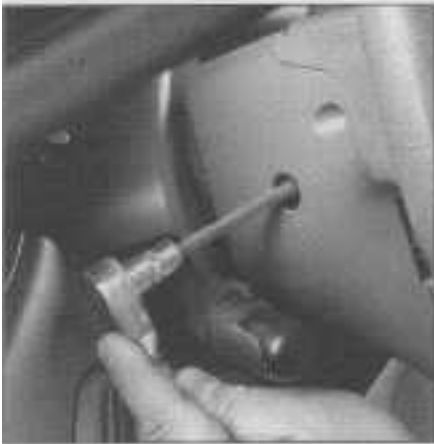
20.3 Remove the two screws retaining the steering wheel airbag module
