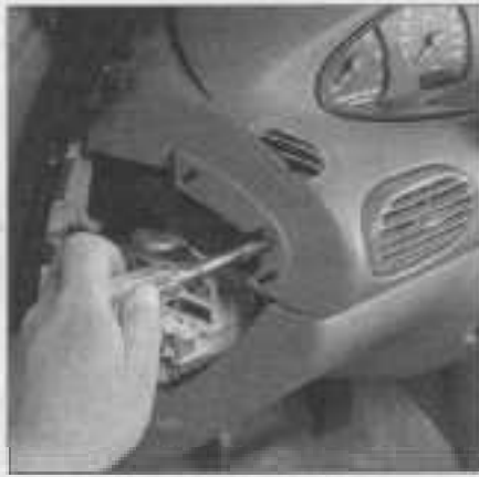
22.3 Removing the screw securing the left side of the instrument cluster hood
