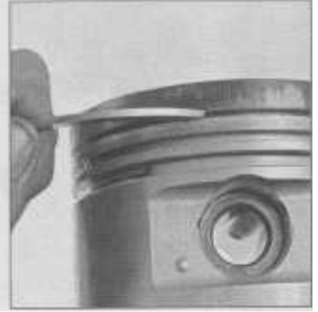
20.4b . . . or a short piece of an old compression ring
