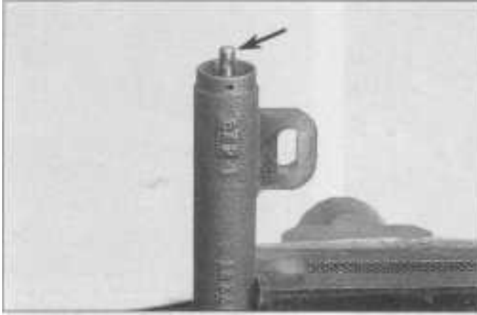
6.32a The hydraulic tensioner piston (arrow) must be compressed into the tensioner housing prior to installation
