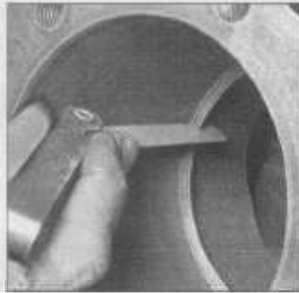
24.4 With the ring square in the cylinder, measure the ring end gap with a feeler gauge
