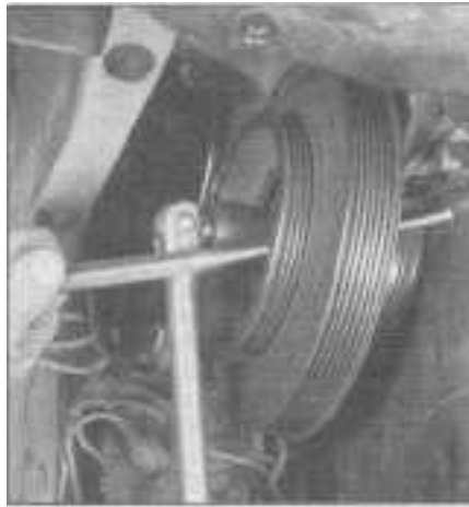
6.4a To keep the crankshaft from turning, insert a large screwdriver or bar through the opening in the damper/pulley and wedge it against the engine block, then loosen the bolt with a socket and breaker bar
