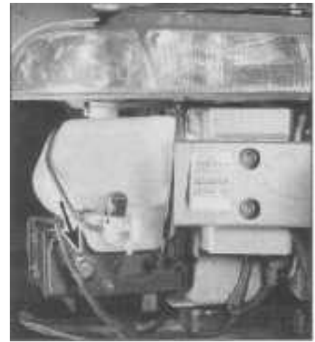
7.12 On 1995 models, the EVAP system charcoal canister (arrow) is located behind the right front bumper fascia (removed for clarity)
