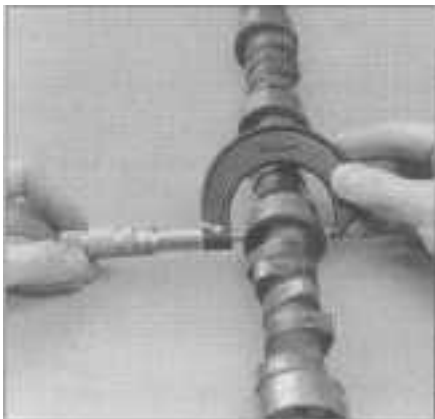
10.12 Measure the camshaft bearing journal diameters with a micrometer and compare the measurements to the dimensions given in this Chapter's Specifications
