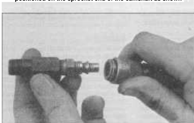
11.5 This is what the air hose adapter that threads into the spark plug hole looks like - they're readily available from auto parts stores
