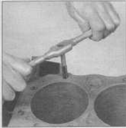
17.8 All bolt holes in the block, particularly the main bearing cap and head bolt holes, should be cleaned and restored with the appropriate tap (be sure to remove the debris from the holes after this operation)
