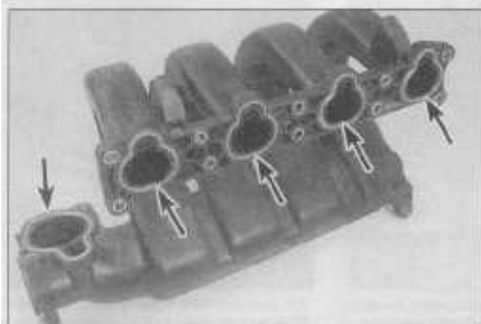
4.13 On 2.0L engines, remove the O-ring seal gaskets (arrows) on the throttle body and intake ports
