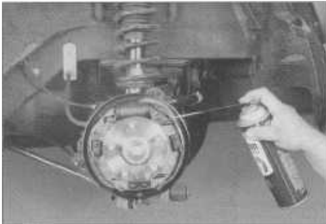
6.2 Before disassembling the brake shoe assembly, spray it with brake cleaner to remove brake dust; DO NOT blow brake dust off with compressed air
