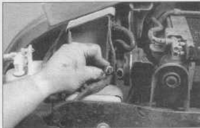
21.9 Lower horn electrical connector
