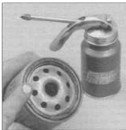
8.18 Lubricate the oil filter gasket with clean engine oil before installing the filter on the engine
