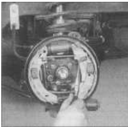
6.4t Install the adjuster spring into the trailing brake shoe, then attach it to the adjuster
