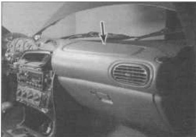
29.1b The passenger's airbag (arrow) is located on the dashboard above the glove box
