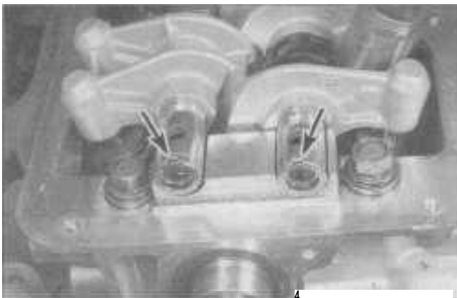
9.19 Both rocker arm shafts must be installed with the notches (arrows) facing UP and at the timing belt end of the engine
