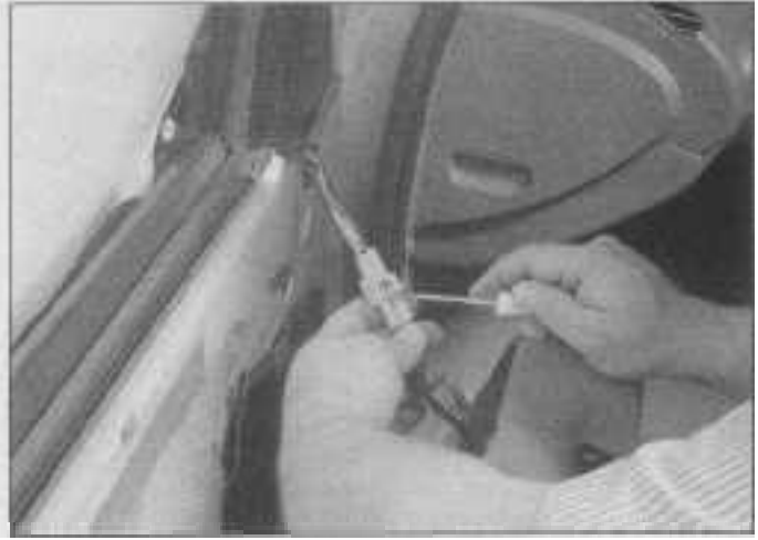
13.11 Disconnect the outside mirror electrical connector from the door trim panel
