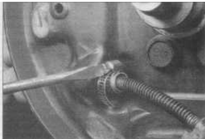
14.13 If a 1/2 inch box-end wrench isn't available, use a small hose clamp to compress the parking brake cable retaining clip tabs
