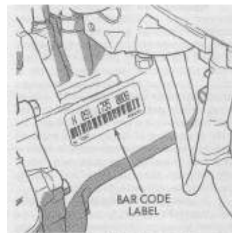
The transaxle identification number can be found on the side of the case (as shown) or the top of the bell housing
