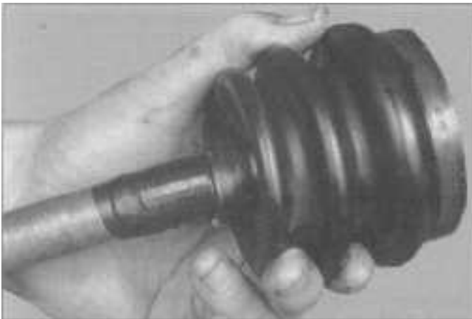
9.10 Before installing the boot, wrap the axle shaft splines with tape to prevent damaging the boot
