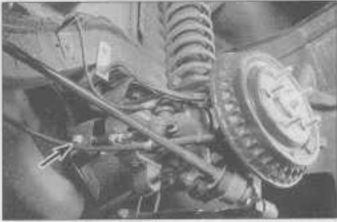
13.4 Remove the front lateral link-to-crossmember bolt (arrow) and nut
