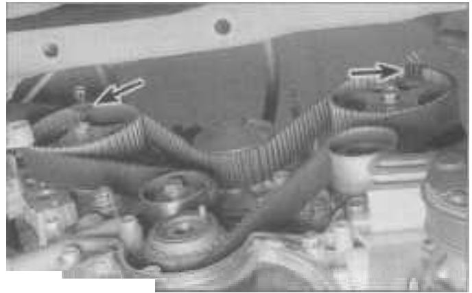
6.22 Binder clips (arrows) can be used to retain the timing belt in position on the camshaft sprockets during installation
