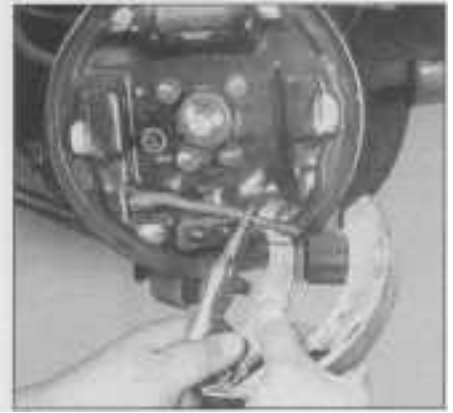
6.4l Obtain the correct replacement trailing brake shoe (they are unique for each side of the vehicle, RH or LH and the parking brake actuating lever should be permanently attached) and install the parking brake cable onto the actuating lever
