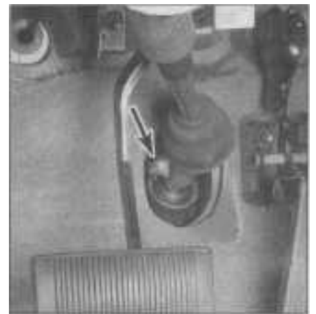
22.3 At the base of the steering column, slide the boot up and remove the retaining pin and pinch bolt (arrow)
