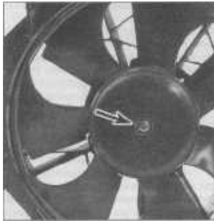
4.9 The fan blade is retained to the motor with either a nut or a clip (arrow)
