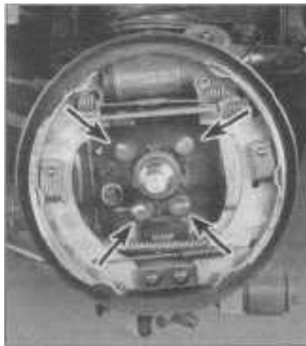
18.5a Remove the brake backing plate bolts (arrows)
