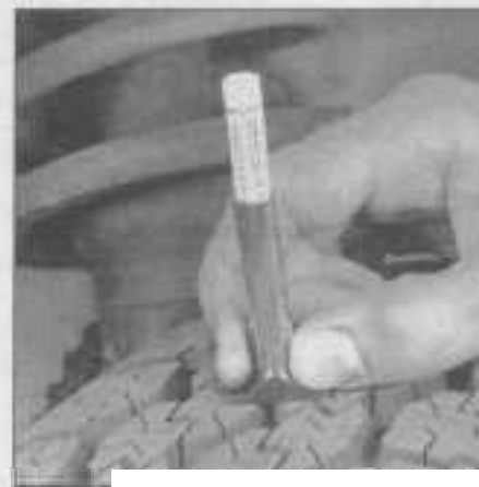
5.2 Use a tire tread depth indicator to monitor tire wear - they are available at auto parts stores or service stations and are relatively inexpensive
