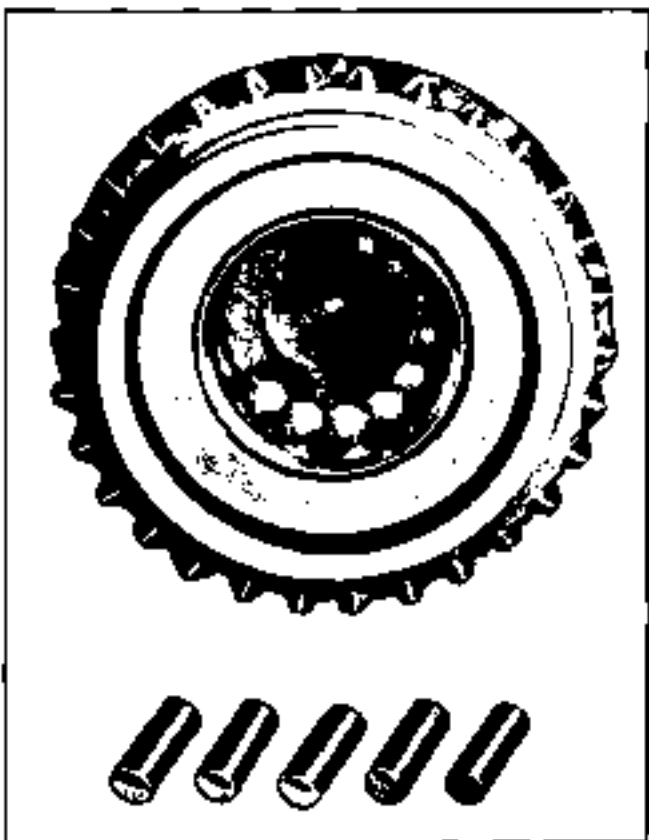
Fig. 7C-16 Loading Bearings into Main Drive Gear
