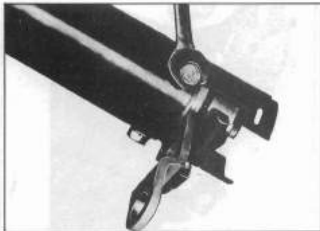
Fig. 9-27 Removing Lower Shift Tube Support Screws Manual Transmission
