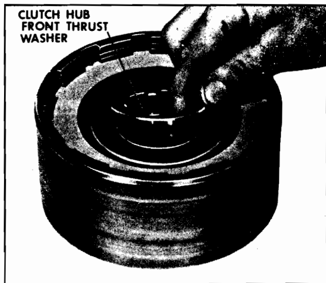
Fig. 7F-50 Removing Clutch Hub Front Thrust Washer
