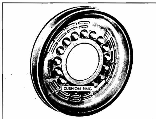
Fig. 7F-95 Reverse Clutch Cushion Ring
