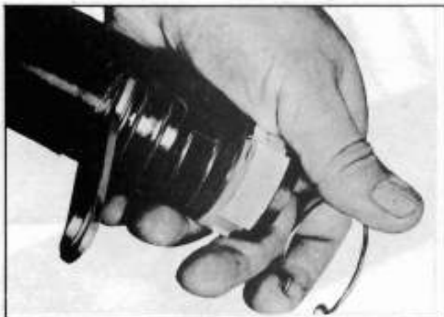
Fig. 9-25 Removing Bearing Adapter and Shift Tube Spring
