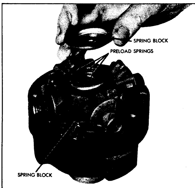
Fig. 4B-15 Installing Second Spring Block - Four Pinion Tempest, Firebird and Grand Prix
