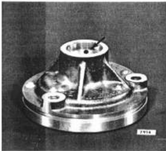
Oil pump body with modified oil return bore
