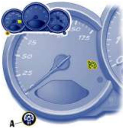
A - Adjustment button for instrument illumination and trip counter
