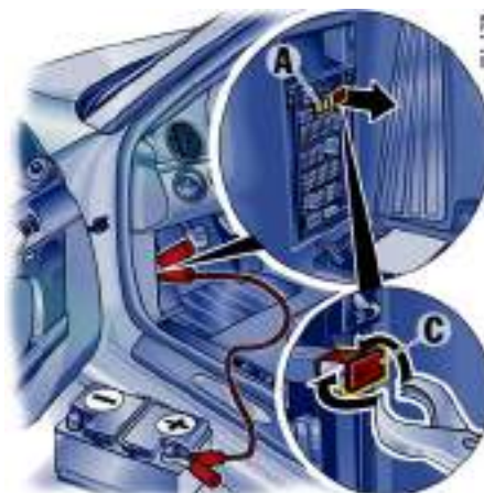
A - Plastic gripper (yellow) C - Positive terminal (red)
