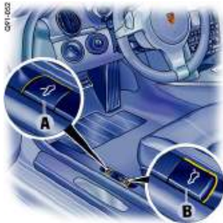
A - Opening front luggage compartment lid B - Opening rear luggage compartment lid
