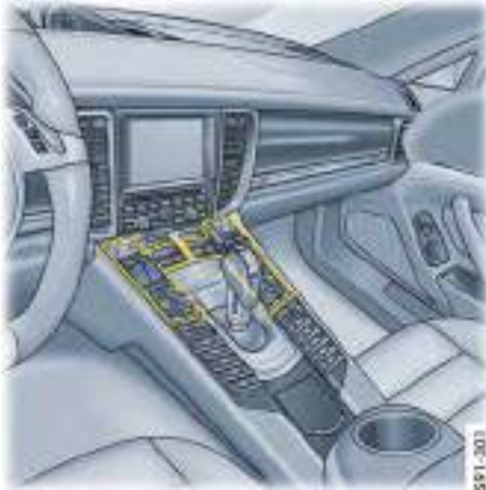
Front air-conditioning control panel
