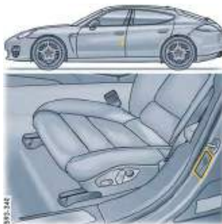
Safety compliance sticker
