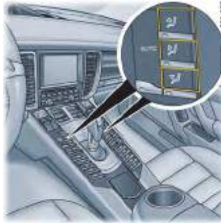
Air distribution, front control panel
