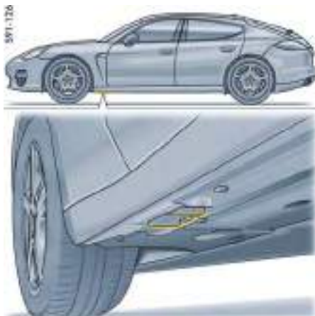
Jacking point for lifting platform and jack at the front
