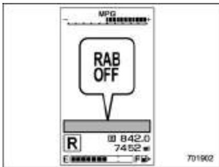
RAB OFF indicator: illuminates when the Reverse Automatic Braking system is turned OFF.
