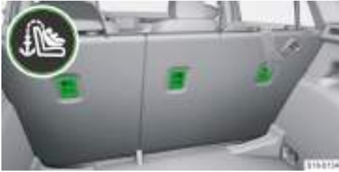
Holding eyelets on the rear seats
