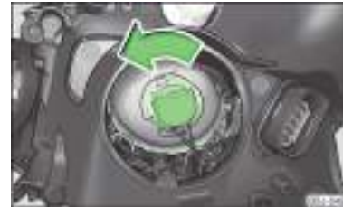
Fig. 163 Removing the bulb for the low beam
