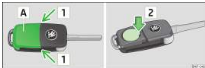
Fig. 27 Remote control key: Remove cover/remove battery
