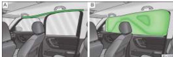
Fig. 11 Location of the head airbag/gas-filled head airbag
