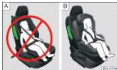
Fig. 16 Incorrect seated position of a child who is not properly secured - risk from the side airbag/Child properly protected by safety seat
