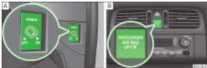
Fig. 12 Key-operated switch for the front passenger airbag / warning light for front seat passenger airbag deactivation
