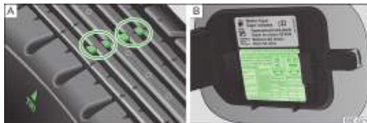
Fig. 141 Principle sketch: Tyre tread with wear indicators/open fuel filler flap with a table detailing the tyre sizes and tyre inflation pressures
