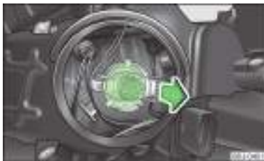
Fig. 162 Removing bulbs for low and main beam
