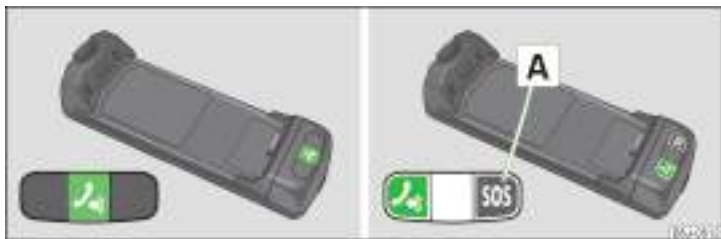
Fig. 105 Principle sketch: Adapter with one button/adapter with two buttons
