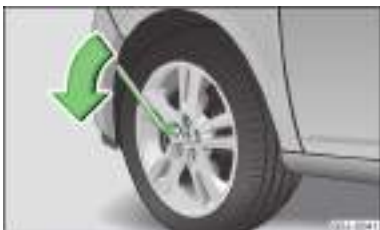
Fig. 148 Changing a wheel: Loosening the wheel bolts
