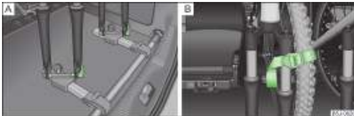
Fig. 74 Put in the bicycle/example fastening the front wheel
