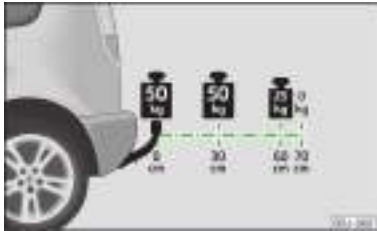
Fig. 129 Representation of the maximum permissible level of the ball head of the towing hitch and the permissible total weight of the accessories including the load depending on the load center of gravity
