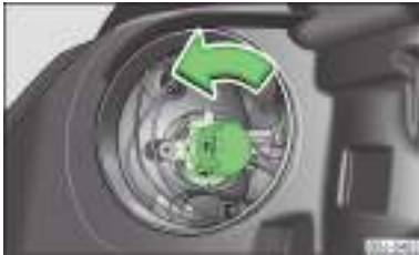
Fig. 164 Removing the bulb for the main beam
