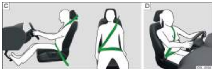
Fig. 6 Routing of belt webbing over the shoulders and the lap belt/Routing of belt webbing for an expectant mother
