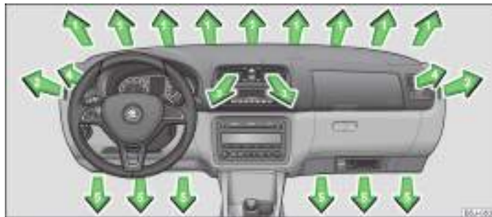
Fig. 99 Air outlet vents
