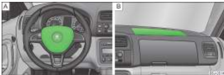
Fig. 8 Driver airbag in the steering wheel/front passenger airbag in the dashboard
