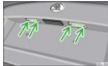
Fig. 168 Remove the licence plate light
