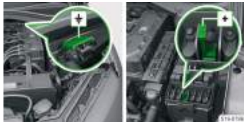
Engine compartment: Earth point and ⊕ pole on vehicles with the battery in the luggage compartment
