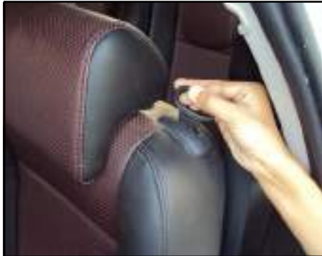
Plastic hook for folding seat backrest
