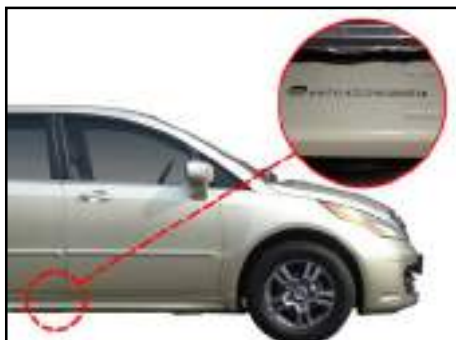
Chassis No. - Punched on RH Long member
