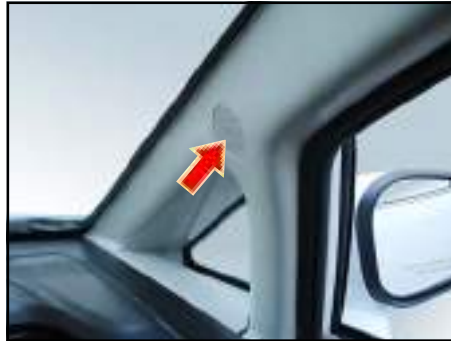
Tweeter located on 'A' pillar
