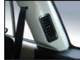
A.C. air vents on 'C' pillar for third row seat
