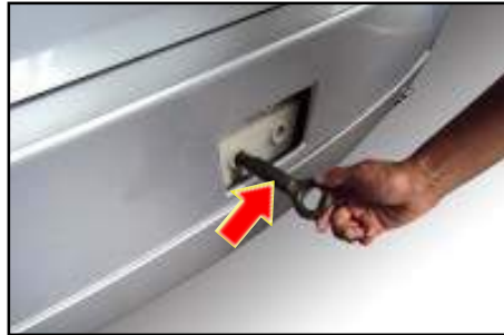
Tow Hook Attachment Location at Rear
