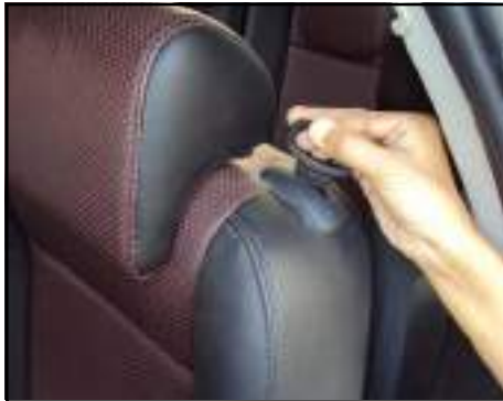
Plastic hook for folding seat backrest
