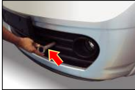
Tow Hook Attachment Location at Front
