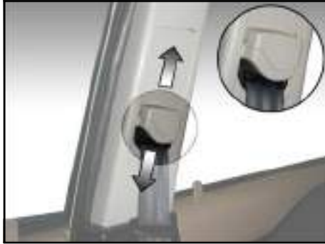
Seat belt height adjustment
