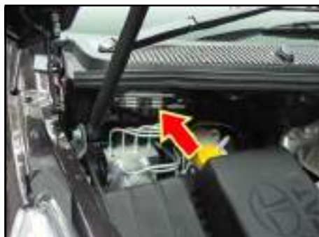
VIN Number Plate (Near ABS Unit)
