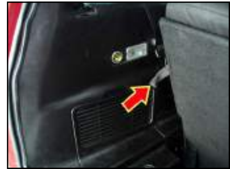
Fabric hook for folding seat backrest
