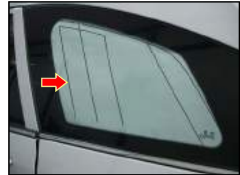
Antenna located on third quarter glass
