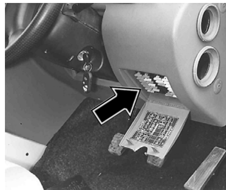
Fuse Box - Cabin
