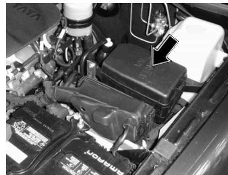
Fuse Box - Engine Compartment
