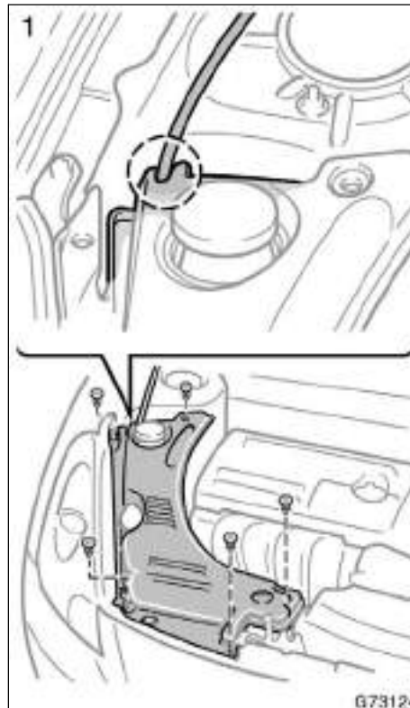
5. RIGHT SIDE HEADLIGHT—Install the cover.
