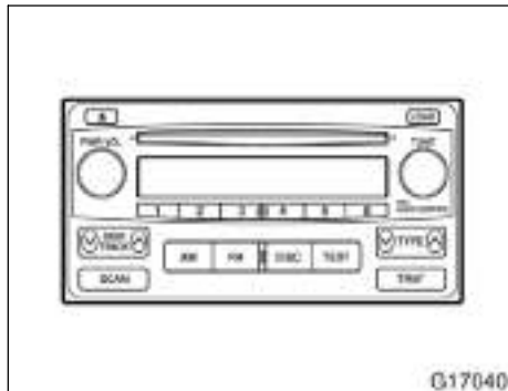
Type 2: AM-FM radio/compact disc player with changer
