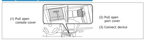
Use this port to connect a portable audio device and listen to it through the vehicle's speakers.
