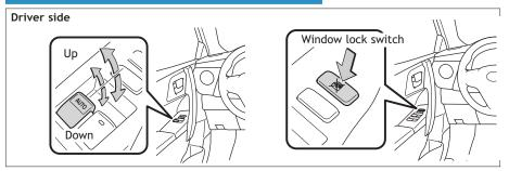
**Automatic operation (driver's window only)** Push the switch completely down and release to fully open. To stop the window partway, operate the switch in the opposite direction.
