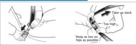
NOTE: If a passenger's seat belt is fully extended, then retracted even slightly, the Automatic locking retractor (ALR) will prevent it from being re-extended beyond that point, unless fully retracted again. This feature is used to help hold child restraint systems securely.
