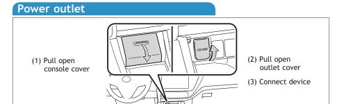
Designed for car accessories. Ignition switch must be in the "ACC" or "ON" position to use.
