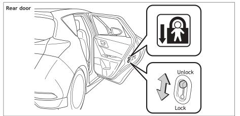
Moving the lever downward will allow the door to be opened only from the outside.
