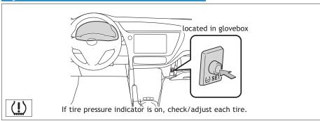
After adjusting tire pressures, or after tires have been rotated or replaced, turn the ignition switch to "ON" and press and hold the "SET" button until indicator blinks three times. Let the vehicle sit for a few minutes to allow initialization to complete.
