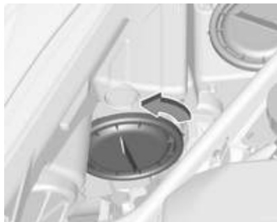
Low beam (1) outer bulb. High beam (2) inner bulb.
