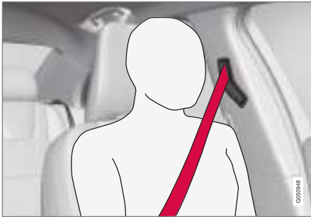
Correctly fitted seatbelt.
