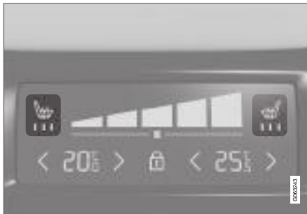
Seat heating indication and controls on the climate panel at the rear of the tunnel console.
