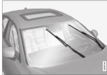
Wiper blades in service position.
