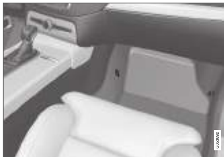
Mounting point locations in the front seat.
