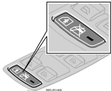
Switch for electric child safety locks and disengaging rear power window buttons.
