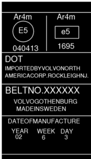
Label on seatbelts with seatbelt tensioner
