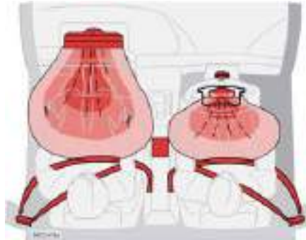
SRS system, right-hand drive.
