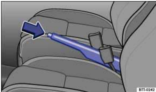
Fig. 103 Between the front seats: Parking brake.
