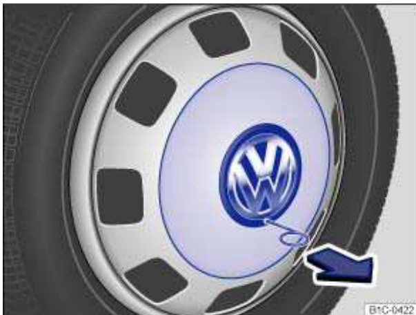
Fig. 140 Pulling the wheel cover off (Version 2).
