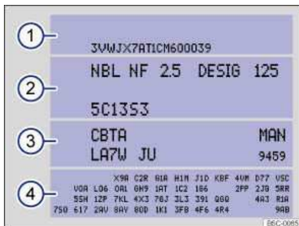
Fig. 15 Vehicle identification label: shown in the example with engine identification code CBTA 3.
