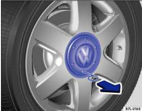
Fig. 171 Pulling the hubcap off.
