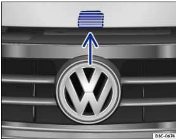
Fig. 142 Above the radiator grille: Outside engine hood release.
