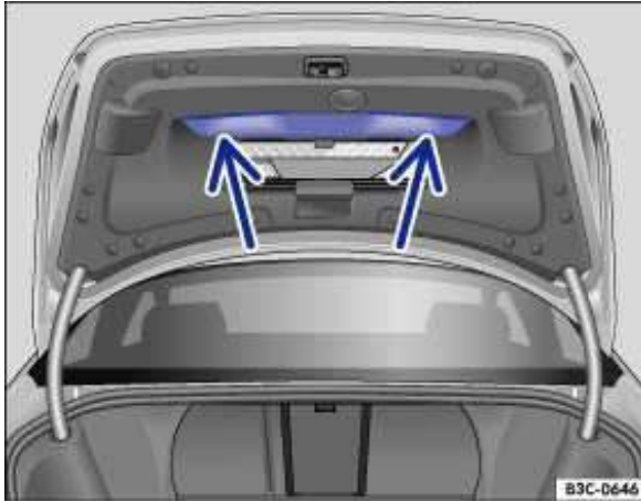
Fig. 26 Opened luggage compartment lid: Recessed grips for closing.
