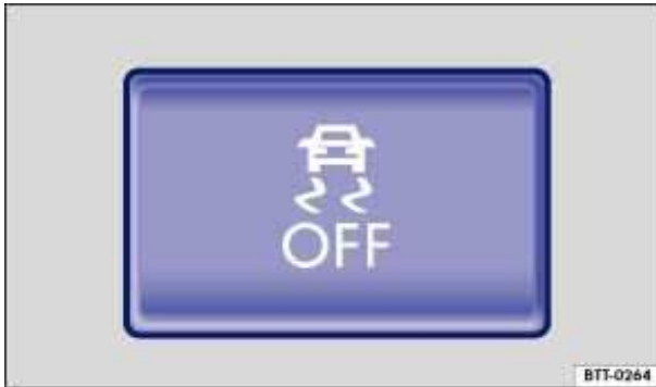
Fig. 122 In the center console: Button for switching ASR on and off manually.
