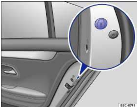
Fig. 162 On the edge of the right rear door: Emergency lock, covered by a rubber seal.
