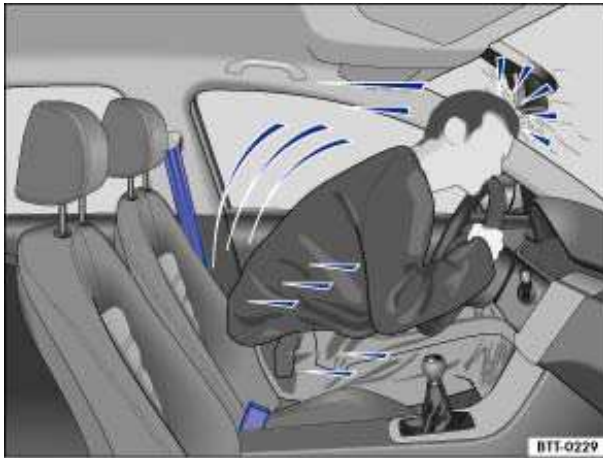
Fig. 49 The unbelted driver is thrown forward.
