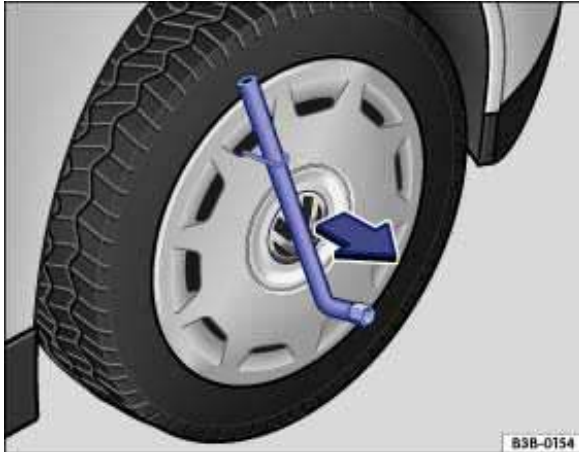
Fig. 173 Pulling the wheel cover off.
