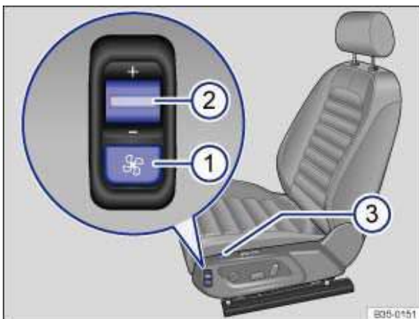
Fig. 44 On front seat: Switch for seat ventilation.
