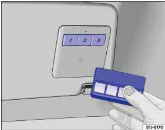
Fig. 29 In the driver side sun visor: The remote control and buttons for the HomeLink Universal Transmitter.
