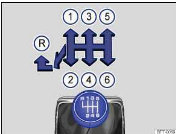
Fig. 116 Gearshift pattern of a 6-speed manual transmission.
