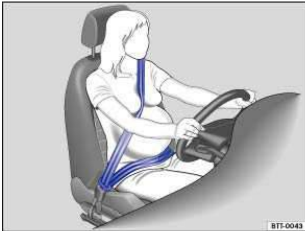
Fig. 55 Proper safety belt positioning for expectant mothers.
