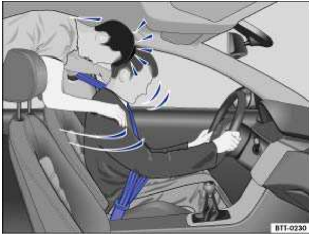
Fig. 50 Unbelted passengers in the rear seats are thrown forward on top of the belted driver.
