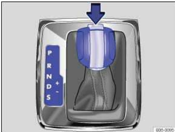
Fig. 118 Automatic transmission selector lever with shift lever release button (arrow).
