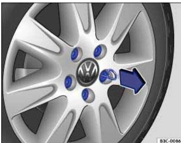
Fig. 174 Pulling cover caps off wheel bolts.
