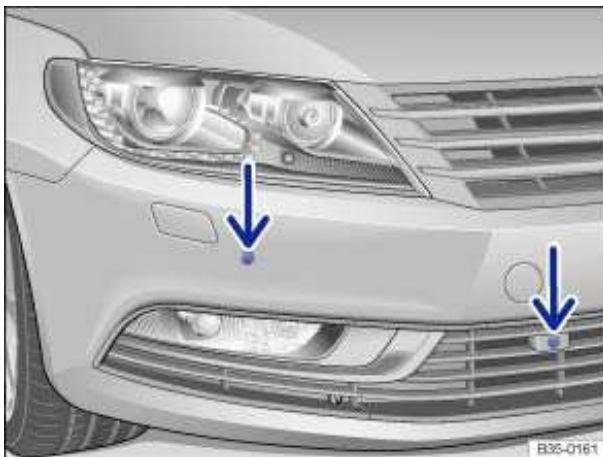
Fig. 127 Park Distance Control system sensors.
