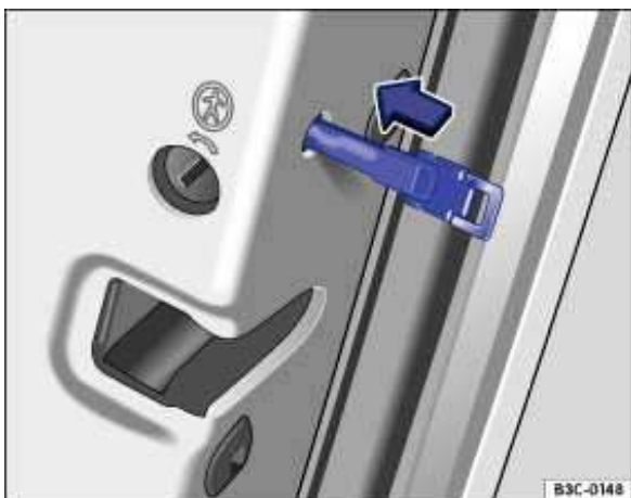
Fig. 163 Locking the vehicle using the emergency key.
