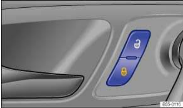
Fig. 21 In the vehicle doors: Power locking button.
