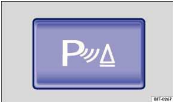
Fig. 126 In the center console: Button to switch the Park Distance Control system on or off.
