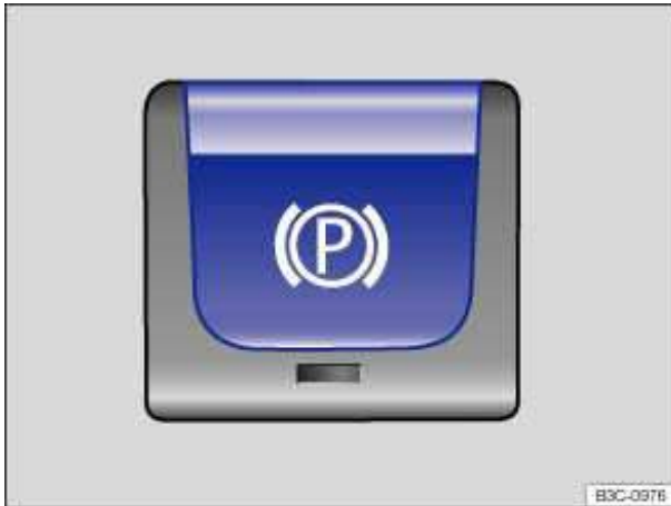
Fig. 121 In the lower section of the center console: Electronic parking brake button.
