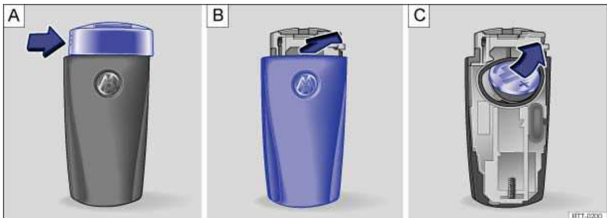
Fig. 19 Remote control vehicle key: Opening the battery compartment cover.
