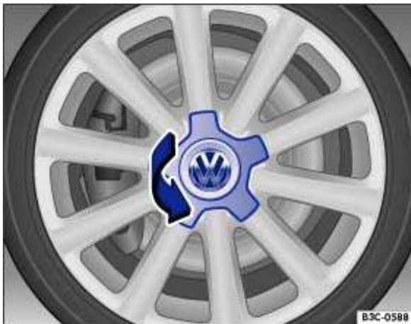
Fig. 172 Twisting the hubcap off.
