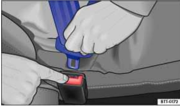
Fig. 53 Releasing the buckle tongue from the belt buckle.
