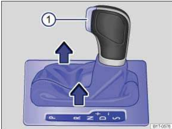
Fig. 167 Removing the selector gate cover.
