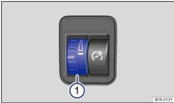
Fig. 74 To the left of the steering wheel: Thumbwheel to adjust instrument panel lighting 1.
