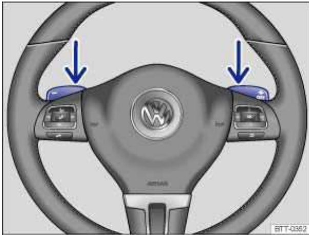
Fig. 120 Steering wheel with optional Tiptronic shift paddles.
