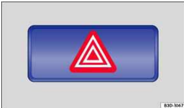
Fig. 160 In the center of the instrument panel: Switch for emergency flashers.
