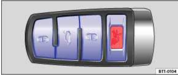
Fig. 16 Remote control vehicle key with panic button.
