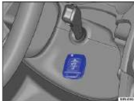
Fig. 126 Hold the remote control vehicle key to the right of the steering column: Emergency starting feature on vehicles with Keyless Access.
