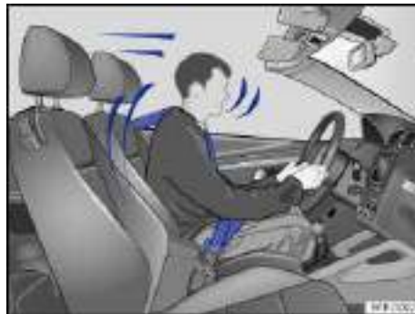
Fig. 58 Belted driver secured by the correctly worn safety belt in the event of a sudden braking maneuver.
