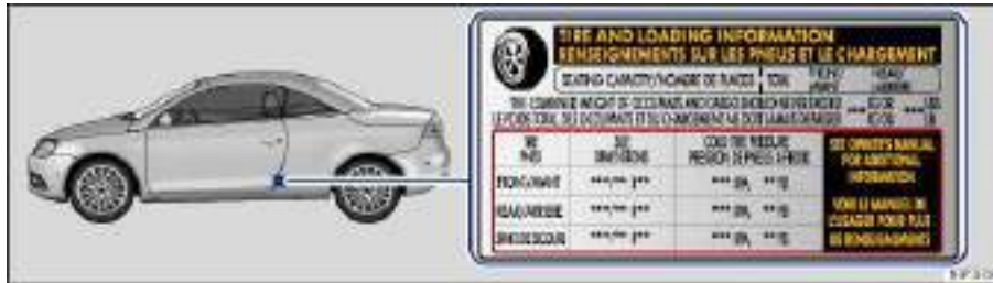
Fig. 104 On the driver door jamb: Location of the tire inflation pressure label.
