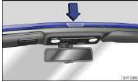
Fig. 36 Wind deflector in the windshield frame.
