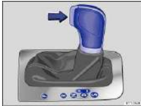
Fig. 128 Side view: Automatic transmission selector lever with shift lever release button (arrow).
