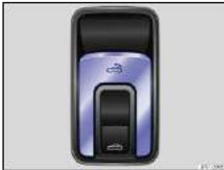
Fig. 32 In the center console: lever for the CSC roof.
