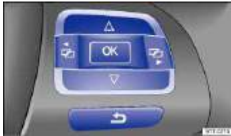
Fig. 15 Right side of the multi-function steering wheel: Controls for menus in the instrument cluster.
