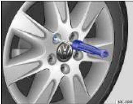
Fig. 187 Changing a wheel: remove previously loosened wheel bolts using the screwdriver handle.
