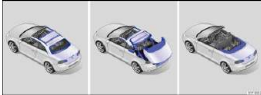
Fig. 31 The CSC roof folds down into the luggage compartment when you open the roof (put the roof down).
