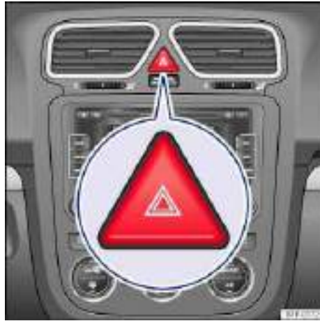
Fig. 163 In the center of the instrument panel: Button for the emergency flashers.
