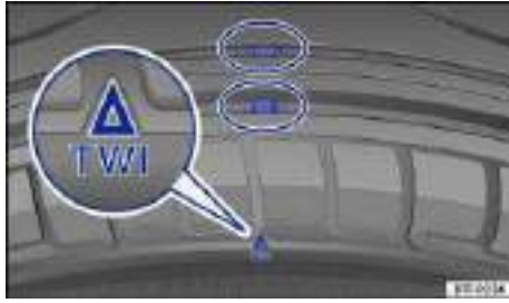
Fig. 105 Tread pattern: Wear indicator.
