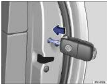
Fig. 166 On the front side of the passenger door: Manual vehicle locking with the key bit in the vehicle key.
