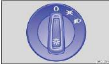
Fig. 75 Headlight switch next to the steering wheel.
