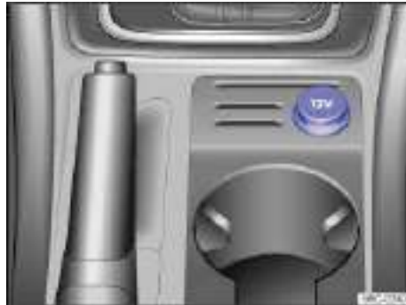
Fig. 124 In the lower center console: 12 Volt socket.
