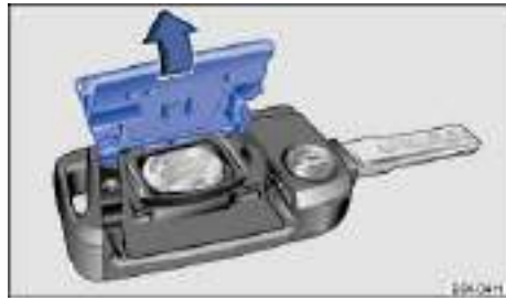
Fig. 20 Remote control vehicle key: Open battery compartment cover.
