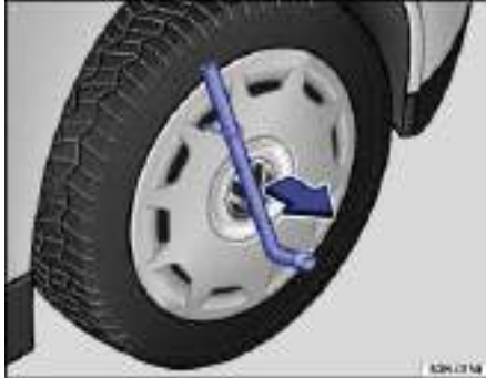
Fig. 190 Pulling the wheel cover off.
