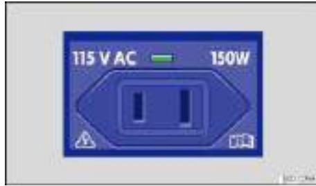
Fig. 126 In the rear center console: 115 Volt outlet with LED display.
