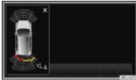
Fig. 152 Mini PDC display of the area surrounding the vehicle.
