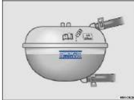
Fig. 170 Coolant expansion tank in the engine compartment.
