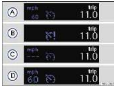
Fig. 143 In the instrument cluster display: Cruise control status indications.
