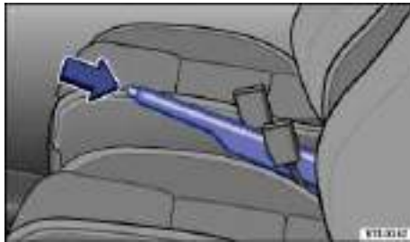
Fig. 139 Between the front seats: Parking brake.
