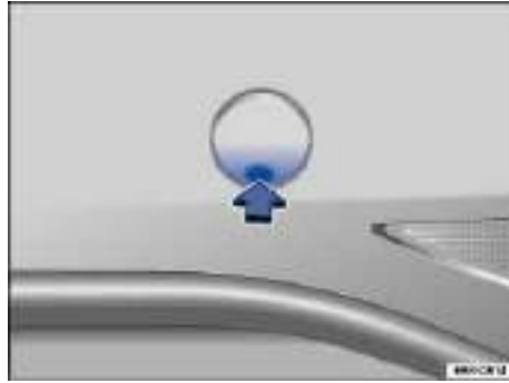
Fig. 204 In the right rear bumper: Removing the cover.
