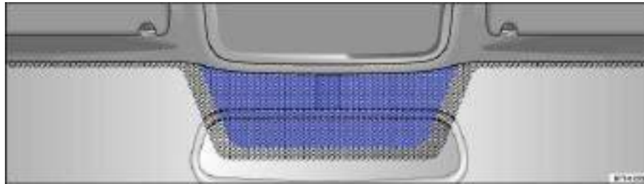
Fig. 79 Heat-reflective windshield with communications window (blue shaded area).
