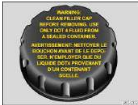
Fig. 140 In the engine compartment: Brake fluid reservoir cap (cap design may vary depending on vehicle equipment).
