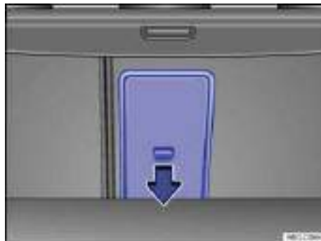
Fig. 95 In the luggage compartment: Opening the pass-through.
