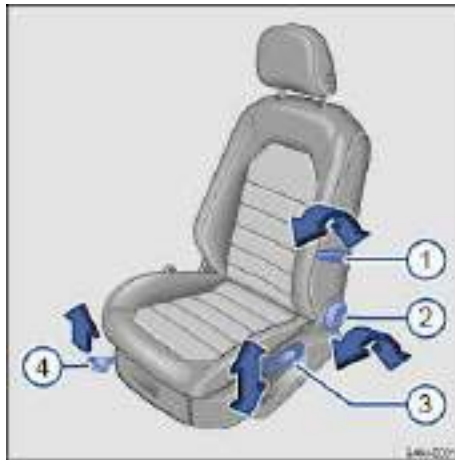
Fig. 36 Driver seat: Manual seat adjustment controls.
