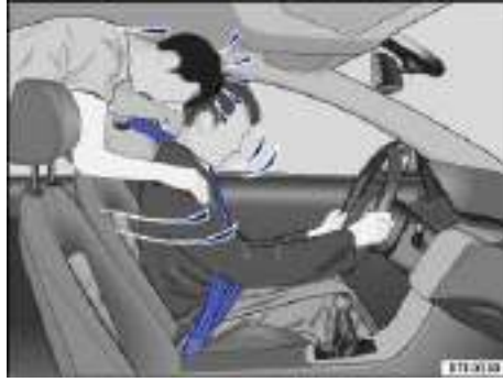
Fig. 52 Unbelted passengers in the rear seats are thrown forward on top of the belted driver.
