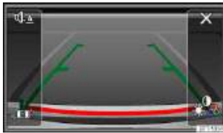
Fig. 146 In the Infotainment system: Rear View Camera system display (display may vary depending on vehicle equipment).
