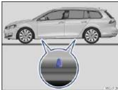
Fig. 192 Lift points for the jack.
