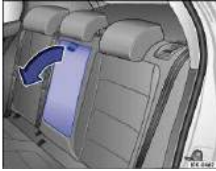
Fig. 46 Folding down the rear center armrest (arrow).
