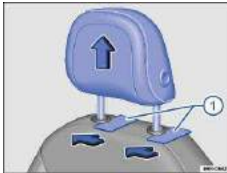
Fig. 41 Removing the front head restraints.
