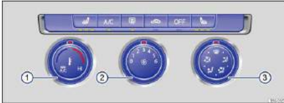
Fig. 157 In the center console: Manual air conditioning controls.
