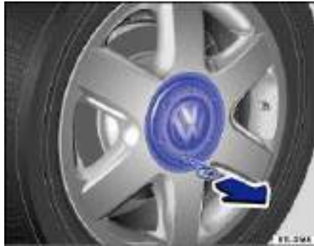
Fig. 187 Pulling the hubcap off.
