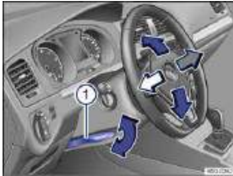
Fig. 44 Manual adjustment for the steering wheel position.
