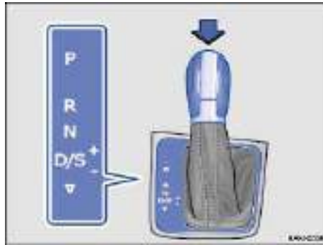
Fig. 135 Automatic transmission selector lever with shift lever release button (arrow).
