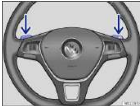
Fig. 137 Steering wheel with Tiptronic shift paddles (if equipped).
