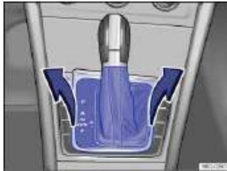
Fig. 182 Removing the selector gate cover.
