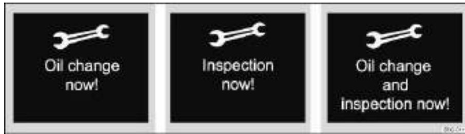
Fig. 12 In the instrument cluster display: Examples of service reminders when a service is due.
