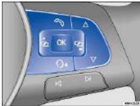
Fig. 14 Right side of the multi-function steering wheel (if equipped): Controls for the menus and information displays in the instrument cluster.
