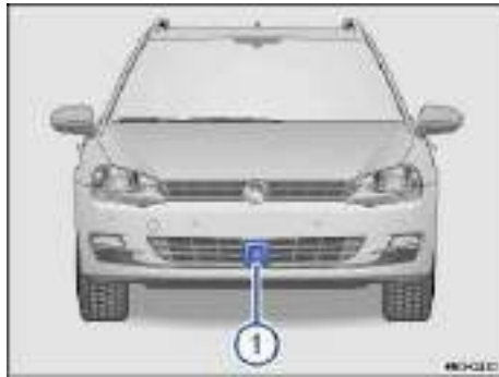
Fig. 155 In the front bumper: Radar sensor.
