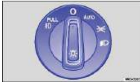
Fig. 76 Headlight switch next to the steering wheel (with fog lights and automatic headlights, if equipped).
