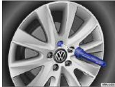
Fig. 195 Changing a wheel: Remove previously loosened wheel bolts using the screwdriver handle.
