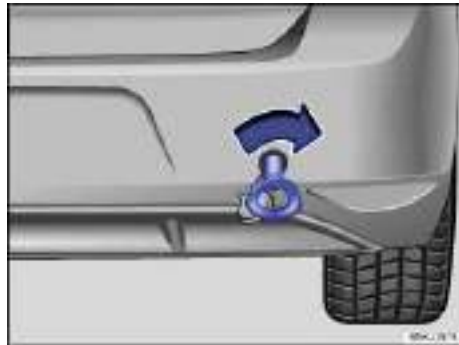
Fig. 205 In the right rear bumper: Installing the towing eye.
