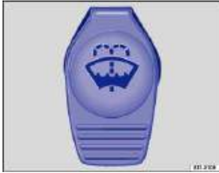
Fig. 85 In the engine compartment: Cap of the windshield washer fluid reservoir.
