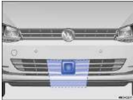
Fig. 156 Area around the radar sensor to be kept clean and free of obstructions.
