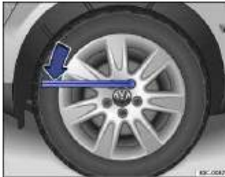
Fig. 191 Changing a wheel: Loosening the wheel bolts.
