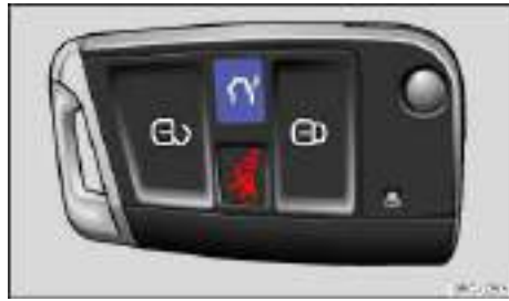
Fig. 28 In the remote control vehicle key: Button to unlock the rear hatch.
