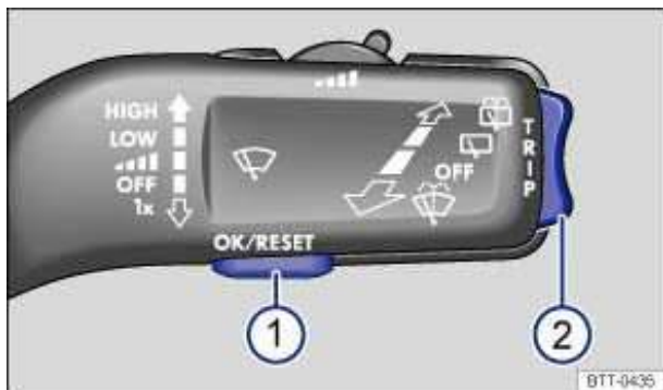
Fig. 15 In vehicles without a multi-function steering wheel: Use button 1 in the windshield wiper lever to confirm menu items and rocker switch 2 to switch menus.
