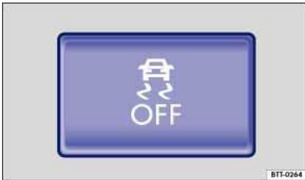
Fig. 137 In the center console: Button for switching ASR on and off manually.
