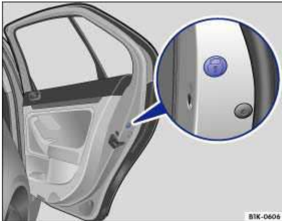
Fig. 174 On the front side of the right rear door: Emergency lock, covered by a rubber seal.
