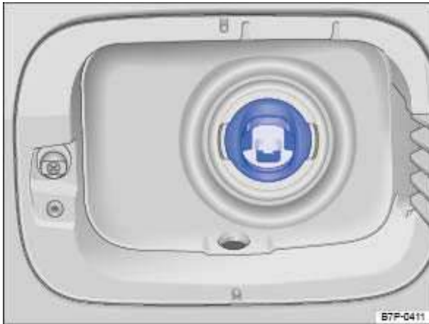
Fig. 152 With open fuel cap: Misfueling guard in the fuel filler neck.
