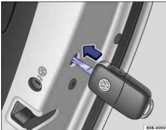
Fig. 175 On the front side of the right rear door: Manual vehicle locking with the key bit in the vehicle key.
