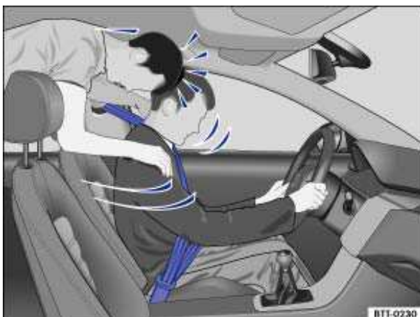
Fig. 53 Unbelted passengers in the rear seats are thrown forward on top of the belted driver.
