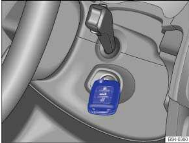
Fig. 127 Emergency starting feature on vehicles with Keyless Access.
