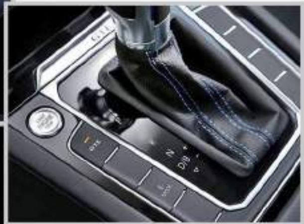
Sport program button (GTE mode) and button for electric drive (E-MODE) next to selector lever
