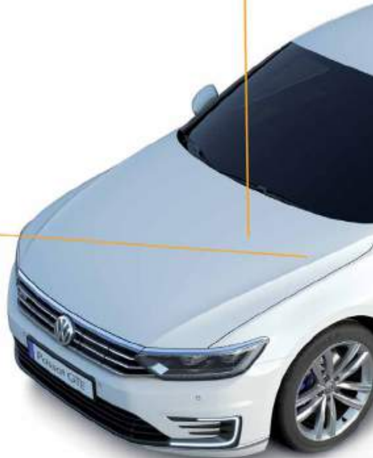
Jump starting point, positive battery terminal
