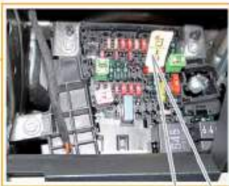
Relay and fuse holder SC at the bottom left of the passenger compartment, behind the storage compartment
