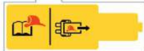
Labelling of emergency cut-out connection in the interior
