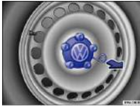
Fig. 188 Pulling off hubcap.
