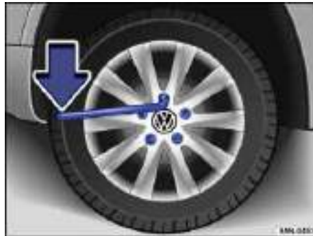
Fig. 191 Changing a wheel: Loosening wheel bolts.
