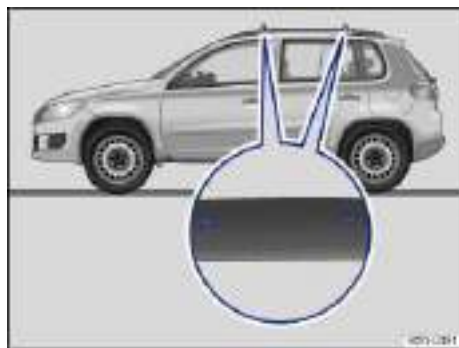
Fig. 108 Vehicles with roof railing: Attachment points for the base carrier and roof rack.
