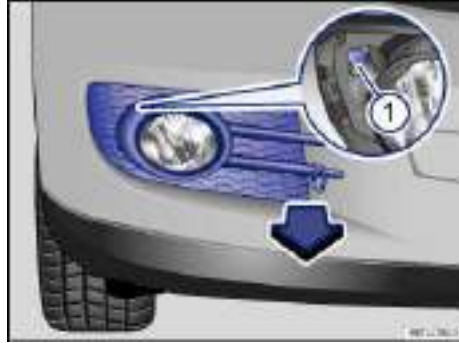
Fig. 202 In right front bumper: Removing light assembly.
