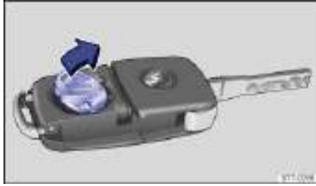
Fig. 24 Remote control vehicle key: Remove old battery.
