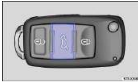
Fig. 31 In the remote control vehicle key: Button to unlock and open the rear hatch.
