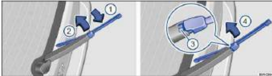
Fig. 172 Changing the rear window wiper blades.
