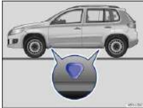
Fig. 192 Lift points for the jack.
