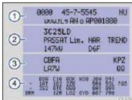
Fig. 18 Vehicle identification label: Shown in the example with engine identification code CBFA 3.
