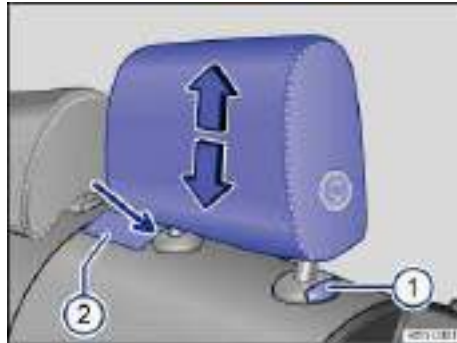
Fig. 49 Removing the rear head restraints.
