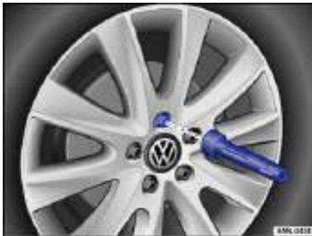
Fig. 194 Changing a wheel: Remove previously loosened wheel bolts using the screwdriver handle.
