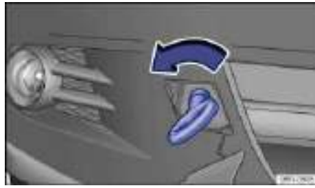
Fig. 211 In right front bumper: Screwing in towing eye.
