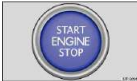
Fig. 135 In the center console: Starter button of the Keyless Access locking and starting system.
