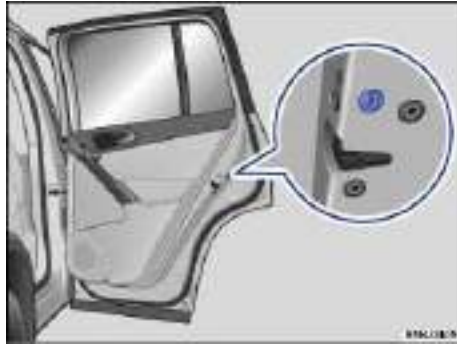
Fig. 179 On the front side of the right rear door: Emergency lock, covered by a rubber seal.
