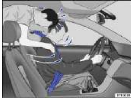
Fig. 61 Unbelted passengers in the rear seats are thrown forward on top of the belted driver.
