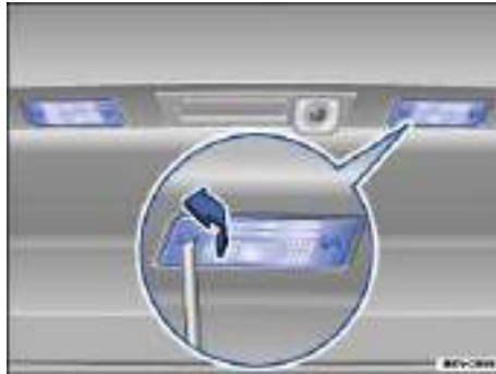
Fig. 209 In the rear hatch: Screwed license plate lamp.
