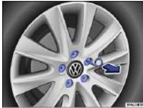
Fig. 189 Pulling cover caps off wheel bolts.
