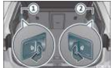
Fig. 129 In the trunk: levers for remote release of the left part ① and right part ② of the rear seat backrest.
