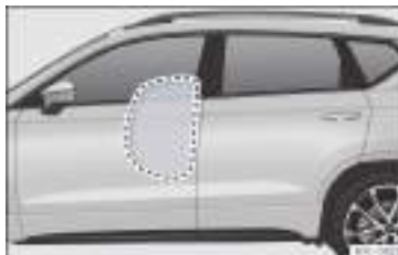
Fig. 27 Illustration of completely inflated side airbags on the left side of the vehicle.
