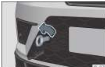
Fig. 64 Right side of the front bumper: towline anchorage screwed in.
