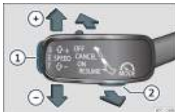
Fig. 205 On the left of the steering column: third lever for operating the speed limiter.
