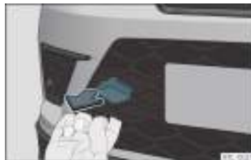
Fig. 84 Front bumper on right: remove the lid.
