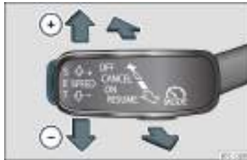
Fig. 44 On the left of the steering column: third lever to operate the CCS.
