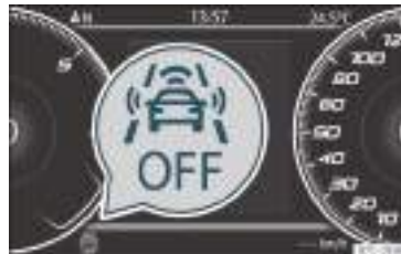
Fig. 208 On the screen of the instrument panel Front Assist switched off message.
