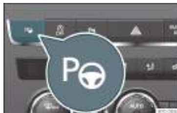
Fig. 226 In the centre console, top section: button to switch on the Park Assist system.
