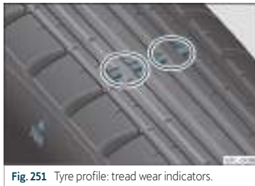
Fig. 251 Tyre profile: tread wear indicators.
