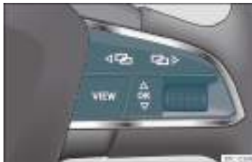
Fig. 105 Right side of multifunction steering wheel: buttons to the menus and informative indications on the instrument panel.
