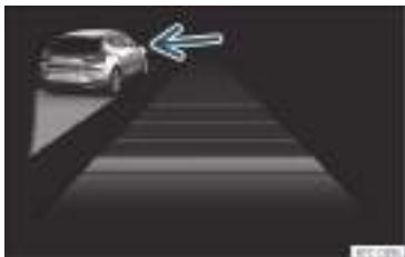
Fig. 214 On the instrument panel display: ACC active, vehicle detected in an outer lane.
