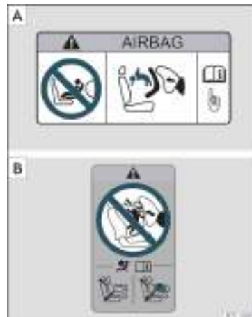
Fig. 30 Airbag adhesives - version 2: on the passenger-side sun blind [A] and on the rear frame of the front passenger's door [B] .
