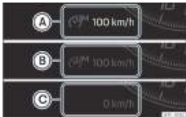
Fig. 203 On the instrument panel display: indications of the speed limiter status.
