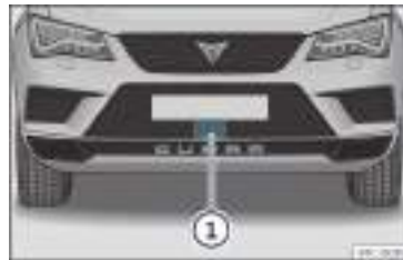
Fig. 211 On the front bumper: radar sensor.
