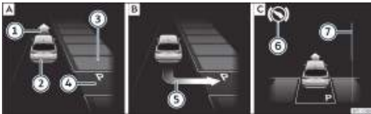
Fig. 230 On the instrument panel display: parallel parking. [A] Finding a parking space. [B] Parking position. [C] Manoeuvring.
