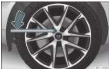
Fig. 61 Wheel: loosen the wheel bolts.
