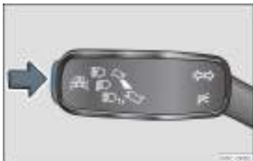
Fig. 106 On the turn light and main beam headlight lever: key for driver assistance systems.
