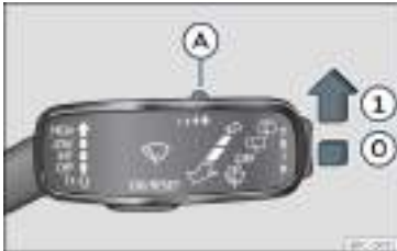
Fig. 123 Windscreen wipers lever: adjust the rain sensor (A).
