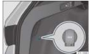
Fig. 134 Detailed view of the side trim in the boot: 12-volt power socket.
