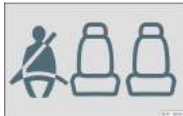
Fig. 75 Dashboard: right rear seat occupied and corresponding seat belt fastened display.
