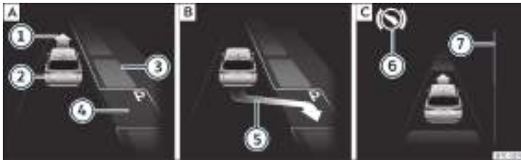
Fig. 229 On the instrument panel display: perpendicular parking. [A] Finding a parking space. [B] Parking position. [C] Manoeuvring.
