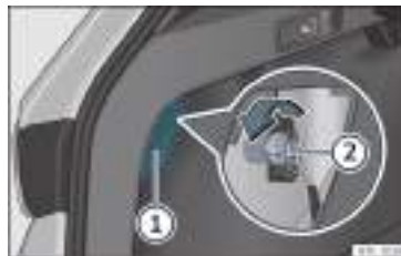
Fig. 91 Boot: access to the bolt securing the tail light unit.
