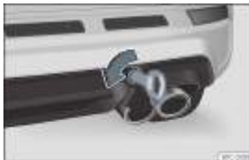
Fig. 87 Right side of the rear bumper: towline anchorage screwed in.
