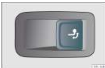
Fig. 243 Right side of the boot: button to unlock the tow hitch.
