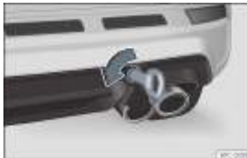
Fig. 65 Right side of the rear bumper: towline anchorage screwed in.
