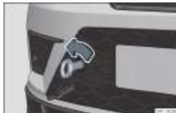
Fig. 85 Right side of the front bumper: towline anchorage screwed in.
