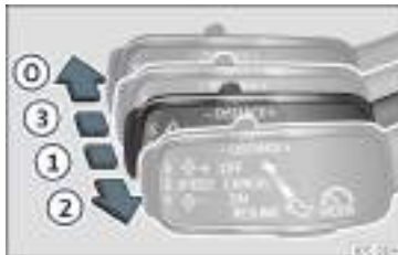
Fig. 212 On the left of the steering column: third lever for operating the Adaptive Cruise Control.
