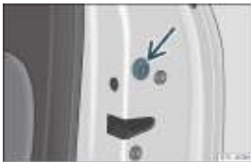
Fig. 4 Locking the door manually.
