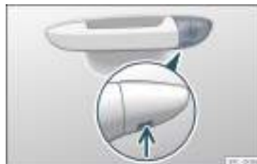
Fig. 3 Driver door lever: hidden lock cylinder.
