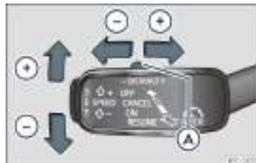
Fig. 213 On the left of the steering column: third lever for operating the Adaptive Cruise Control.
