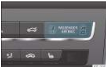
Fig. 82 Dashboard: control lamp for deactivated front passenger airbag in centre console.
