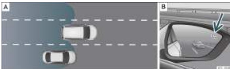
Fig. 223 Schematic diagram: [A] Situation of passing and then moving into the right-hand lane. [B] Indication from the blind spot detector in the right-hand external mirror.
