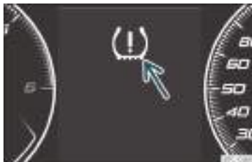
Fig. 253 Instrument panel: warning of loss of tyre pressure.
