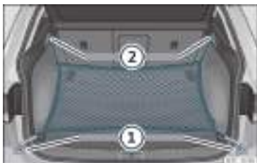
Fig. 144 In the boot: rings ① and hooks ② for attaching the net bag.
