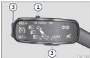
Fig. 204 On the left of the steering column: control and buttons to operate the speed limiter.
