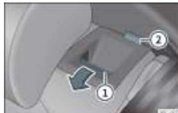
Fig. 128 On the rear seat backrest: release button ①; red mark ②.
