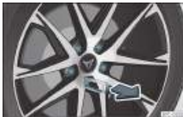
Fig. 59 Wheel: wheel bolts with caps.
