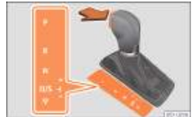
Fig. 56 Automatic transmission: selector lever positions.
