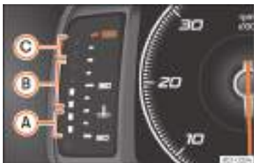
Fig. 135 Digital instrument panel: engine coolant temperature display.
