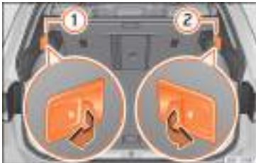
Fig. 164 In the trunk: levers for remote release of the left part ① and right part ② of the rear seat backrest.
