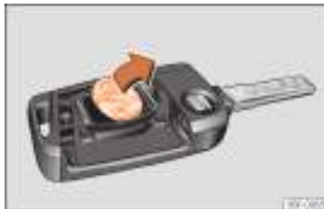
Fig. 146 Vehicle key: removing the battery.
