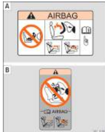
Fig. 36 Airbag adhesives - version 1: on the passenger-side sun blind A and on the rear frame of the front passenger's door B .
