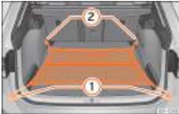
Fig. 189 In the boot: net bag hooked up at floor level (LEON ST model).
