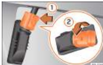
Fig. 122 Number plate light: detach the bulb holder.
