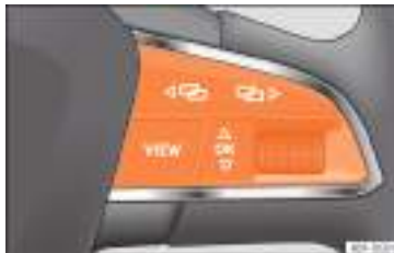
Fig. 137 Right side of multifunction steering wheel: buttons to the menus and informative indications on the instrument panel.
