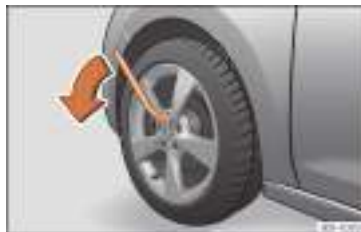
Fig. 77 Wheel: loosen the wheel bolts.
