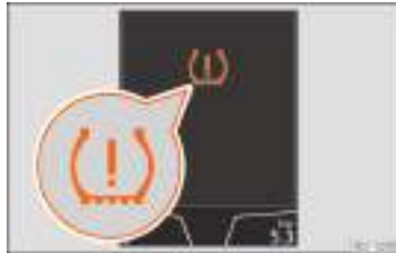
Fig. 315 Instrument panel: warning of loss of tyre pressure.
