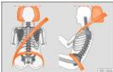
Fig. 22 Correct seat belt and head restraint positions, viewed from front and the side.
