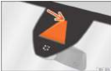
Fig. 277 On the windshield: field of vision of the Lane Assist system camera.
