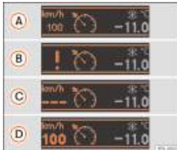
Fig. 264 Instrument panel display: CCS status indications.
