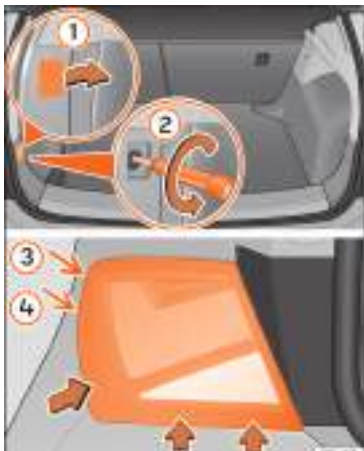
Fig. 115 Trunk: location of the bolt securing the tail light unit. Remove the rear light unit from side panel.
