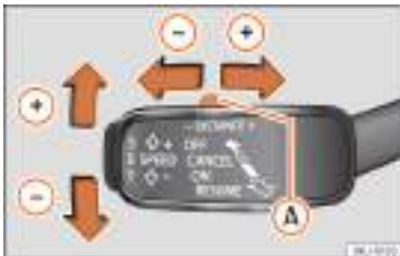
Fig. 273 On the left of the steering column: third lever for operating the Adaptive Cruise Control.
