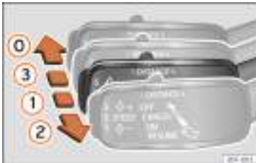
Fig. 272 On the left of the steering column: third lever for operating the Adaptive Cruise Control.
