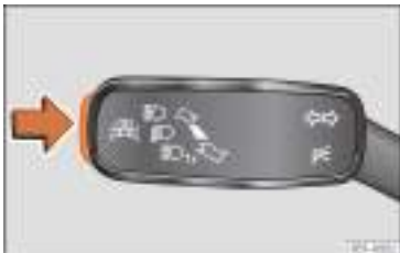
Fig. 138 On the turn light and main beam lever: key for driver assistance systems.
