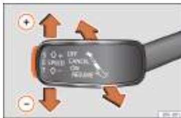
Fig. 54 On the left of the steering column: third lever to operate the CCS.
