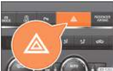
Fig. 152 Dashboard: switch for hazard warning lights.
