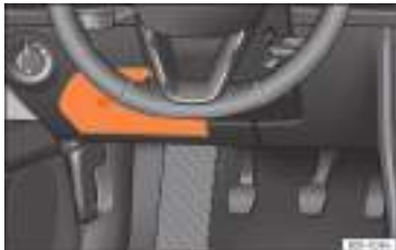
Fig. 67 On the dashboard on the driver side: lid of the fuse box.
