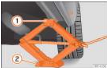
Fig. 79 Crossbar: mounting the jack on the vehicle.
