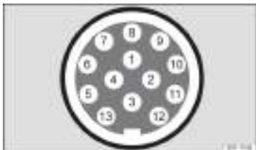
Fig. 302 Diagram: assignment of the pins of the trailer's electrical socket.
