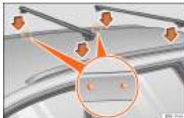
Fig. 196 Leon ST: attachment points for the roof railings for the roof carrier system.
