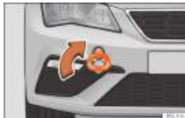
Fig. 101 Right side of the front bumper: towline anchorage screwed in.
