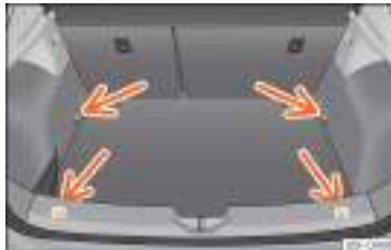
Fig. 185 In the boot: fastening rings (LEON model except versions with spare wheel and CNG).
