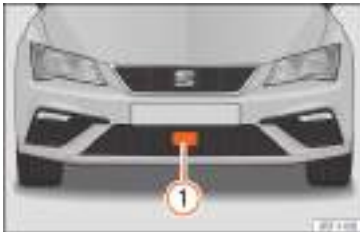
Fig. 266 On the front bumper: radar sensor.
