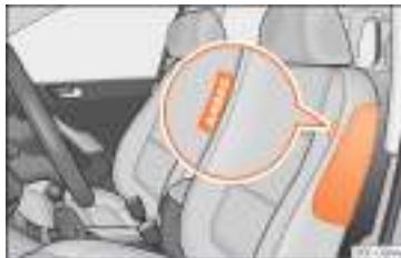
Fig. 32 Side airbag in driver's seat.
