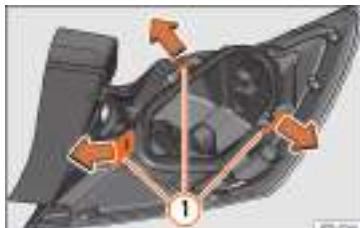
Fig. 116 Retaining tabs on reverse side of tail light.
