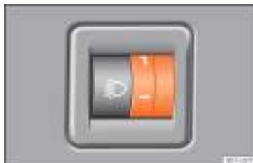
Fig. 153 Next to the steering wheel: regulator headlight range control.
