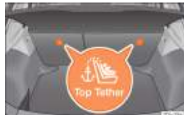
Fig. 41 Position of the Top Tether rings on the back of the rear seat.
