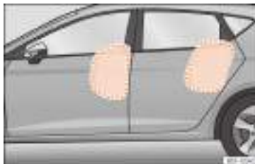
Fig. 33 Illustration of completely inflated side airbags on the left side of the vehicle.
