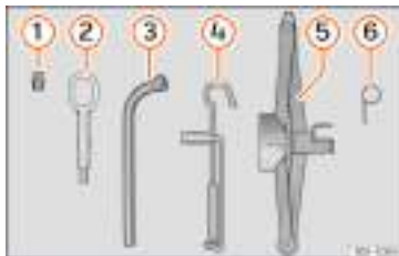
Fig.73 Underneath the floor panel of the luggage compartment: on-board tools.
