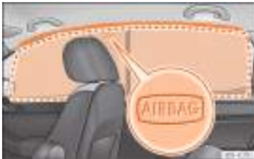
Fig. 34 Location of head-protection airbags.
