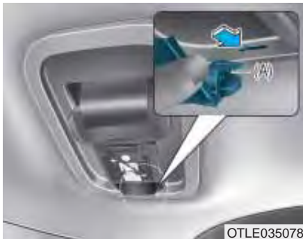
4. Insert the tongue plate (A) into the hole on the belt assembly cover.
