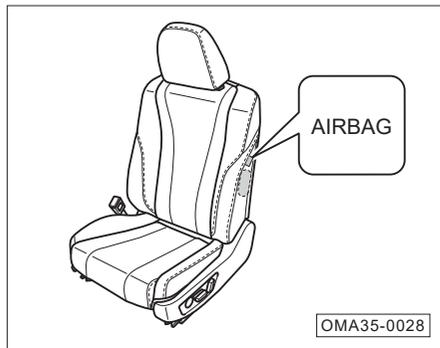
The front seat side airbags are installed in the outboard sides of the driver's seat back and the front passenger's seat back respectively (as indicated by the dotted dash) marked with "SRS AIRBAG".
