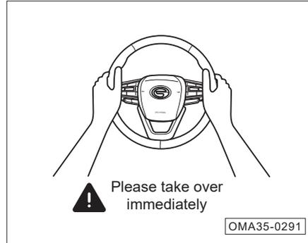
When the LDW detects that the steering wheel is out of the driver's hands for a long time, the system will issue a hands-on reminder and the instrument cluster displays an alarm message while beeping.
