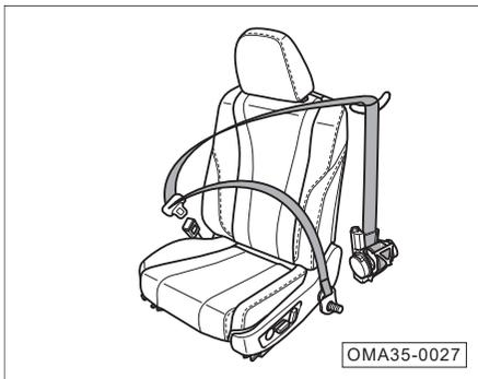
In the event of a vehicle collision, the seat belt, if fastened correctly, can restrain the driver and passengers in a proper position and slow down the inertia of their forward movement, thus preventing them from being thrown forward, and at the same time allow airbags to give them the best protection, thus reducing their impact injury as much as possible.
