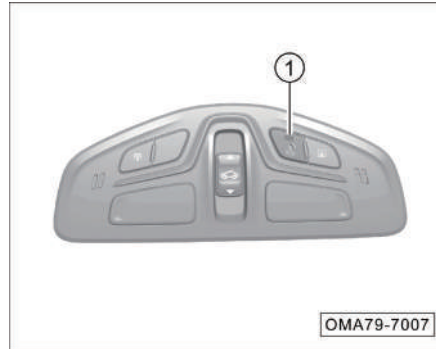
Emergency contact button
