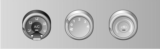
Start the vehicle and turn the front blower control knob to the desired position and press the A/C switch. The indicator on the switch will illuminate, indicating that air conditioning system has been turned on.
