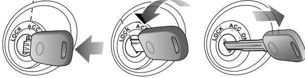
To remove the key from the ignition switch, turn it anticlockwise to position 'ACC'. Then press the key in towards the ignition switch and continue to turn anticlockwise to position 'LOCK'. The key can now be removed.
