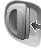
To open the door from the outside, pull the handle and slide the door rearwards.
