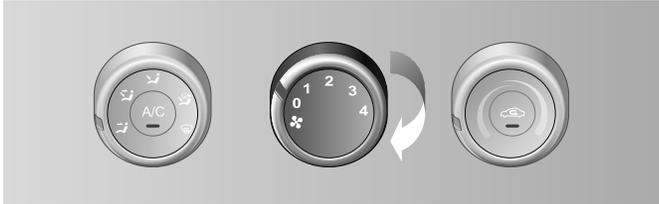
Turn the control knob clockwise and select any position in all four positions to adjust the air quantity at the front vents.
