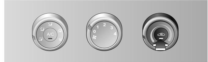
The indicator on the switch will illuminate when the recirculation switch is pressed, indicating that the interior recirculation is started. Press the switch again to start the exterior recirculation. The interior recirculation can also be used if you require a quick warm-up or cool-down of the interior air.
