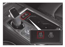
A USB storage device, an external music and video player such as iPod/iPhone/iPad, an MP3 player can be connected to the vehicle through the USB port (type C).
