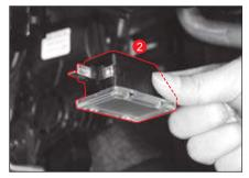
Remove the cover (4) by lifting up the 4 parts on the cover fixing part of the foot lamp assembly (3).
