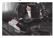
Frequently check the washer fluid level and add the specified product as needed.
