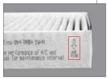
7 After replacing it, install it in the reverse order of A/C filter removal.
