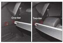
The luggage upper cover can be fixed at the position of one-tier or two-tier according to the angle adjustment level of the rear seat backrest.
