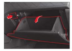
Pull the fixing holder on the left side and the right side of the glove box in the arrow direction.
