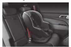
Secure the child restraint with a seat belt as shown in the figure.
