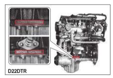
**Diesel Engine:** The engine number is stamped on the bottom surface of the cylinder block behind the exhaust manifold.
