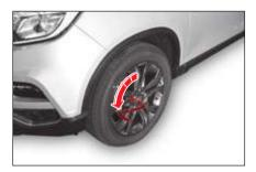
1 Chock the front and rear of the wheel diagonally opposite to the wheel being changed.
