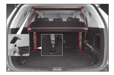
This net prevents the items in the luggage compartment from being thrown in the passenger compartment in an accident.
