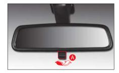
The inside rearview mirror can be adjusted up, down or side ways to obtain the best view by holding the body of the mirror with your hand.
