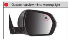
When the outside rearview mirror warning light blinks twice with the START/STOP switch in the ON status or while the engine is running, it indicates that the rear and side warning system is operating normally.
