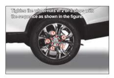
7 Then mount the spare tire and temporarily tighten the wheel nuts until the spare tire wheel is no longer loose.
