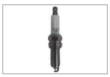
Spark plugs should be inspected periodically for carbon deposits. When carbon accumulates on a spark plug, a strong spark may not be produced.
