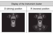
When the obstacle detection sensor is abnormal, "?" is displayed for the relevant sensor. If this message is display on the display of the instrument cluster, have your vehicle checked and serviced at a nearby KG Mobility authorized service center.
