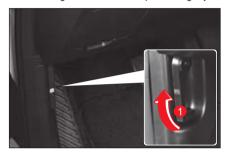
With the engine hood lifted slightly, push the engine hood fixing lever (2) in the arrow direction.
