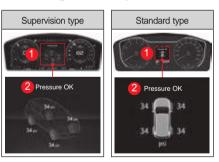
By selecting TPMS status from the main menu (1) of the instrument cluster, you can check all tire pressures from the display (2) of the instrument cluster.
