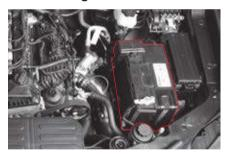
When the battery charge warning light ( ) on the instrument cluster comes on, the battery is not normally charging. If the warning light comes on while driving, turn off all unnecessary electrical devices and have the system checked by a KG Mobility Dealer or KG Mobility Authorized Service Center.
