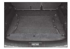
Any loose objects can be stowed securely using the luggage net. Hook the net up to the luggage compartment.
