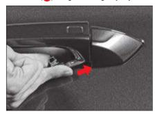
With the Emergency key hole cover open button (1) pressed, push down the top side of the emergency key hole cover to remove it.
