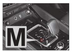
You can shift the gear manually (1st~7th) just as a manual transmission by moving the gear shift lever from the D (driving) position to the M (manual) position.
