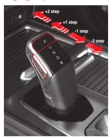
The electronic shift lever can be moved at + 2 step and - 2 step, after which it is always aligned to the central position.
