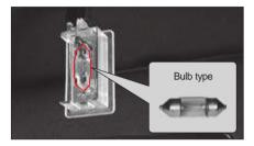
3 After replacing it, install the cover again.
