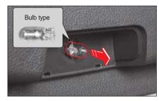
After replacing it, install the cover again.
