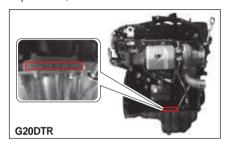
**Gasoline Engine:** The engine number is stamped on the bottom surface of the cylinder block behind the intake manifold.
