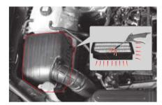
Blow the compressed air through the element in the opposite direction to normal air flow to clean the element as shown above.
