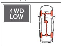
Use the 4WD LOW (4H) mode when the maximum traction power is necessary.
