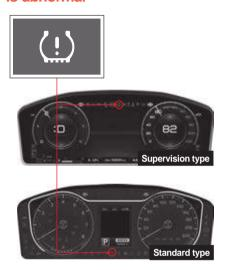
If the tire pressure or the tire pressure monitoring system is abnormal, the global warning light blinks or comes on
