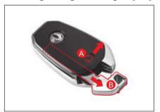
Remove the emergency key (B) from its body while pressing the emergency key lock (A) at the smart key in the direction of the arrow.
