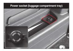
The power socket (12 V/10 A, 120 W) is provided in the vehicle to enable the use of a separate electrical device.
