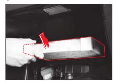
6 Replace it with a new one. Install it with the "AIR FLOW arrow" facing down.
