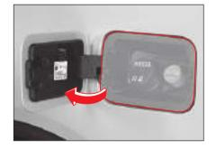
Open the fuel inlet cap by turning it counterclockwise.
