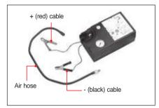
Connect the air hose to the compressor in the service kit.
