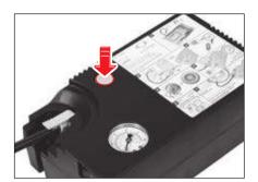
When the prescribed pressure is reached, press the power switch (1) of the service kit to turn it off.
