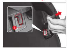
Press the Emergency key hole cover open button (1) using the emergency key.
