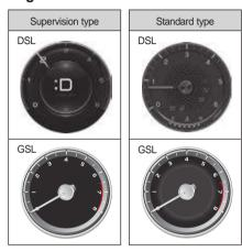
It indicates the revolutions of the engine per minute. Multiplying the number pointed to by the needle by 1,000 is the current engine RPM.
