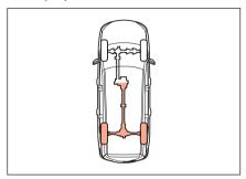
The 2WD (2H) mode is the status for 2WD high speed driving. Use this mode for normal or a high speed driving on a normal road or an expressway.
