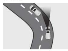
On a curved road, a front vehicle on the same lane cannot be detected and the AEBS performance is reduced so that unnecessary warning or braking is applied or the system may not operate.
