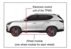
The electronic control unit of the TPMS receives. various data including the tire pressure and temperature from the wheel module mounted on each wheel and displays such data on the instrument cluster.
