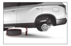
Take the wheel off and place the wheel under the vehicle body. This helps to minimize any danger if the jack slip off position.
