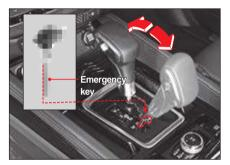
If the gear shift lever cannot be moved from the P (parking) to another position even if the START/ STOP switch is in the ON status and the brake pedal is depressed, move the gear shift lever manually as follows.
