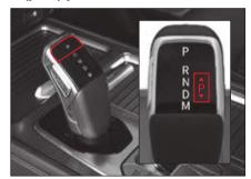
Select this position to park, start the engine, warm-up, and stop the vehicle for a long time.
