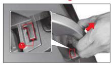
Press the Emergency key hole cover open button (1) using the emergency key.
